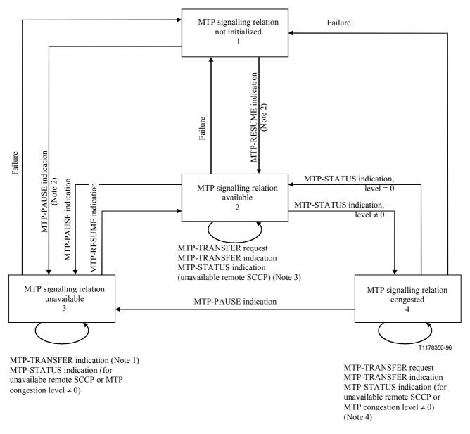
NOTE 1 – MTP-TRANSFER indication in state 3 is a result of the availability of the signalling relation towards the local MTP, but the unavailability of the signalling relation towards the remote MTP.
