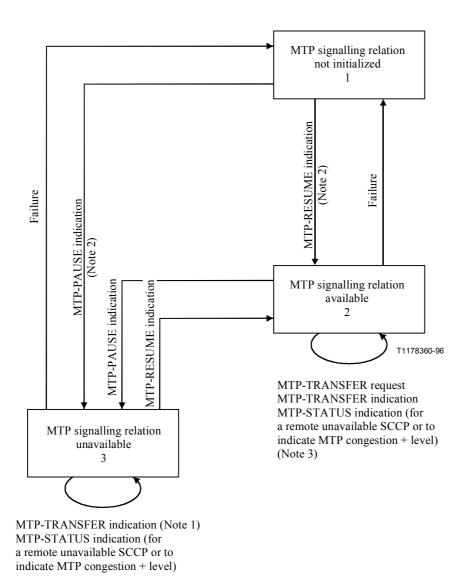
NOTE 1 – MTP-TRANSFER indication in state 3 is a result of the availability of the signalling relation towards the local MTP, but the unavailability of the signalling relation towards the remote MTP.
