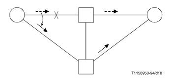
Figure 11/Q.704 – Example of changeover to a signalling route not passing through the remote signalling point
