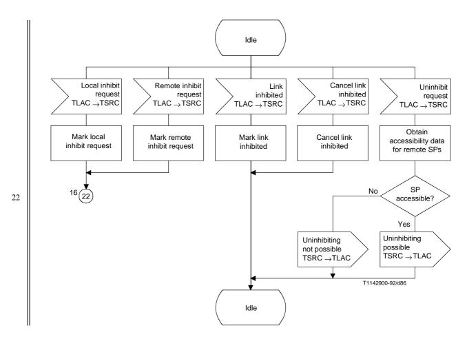
Figure 29/Q.704 (sheet 15 of 21) – Signalling traffic management; signalling routing control (TSRC)
