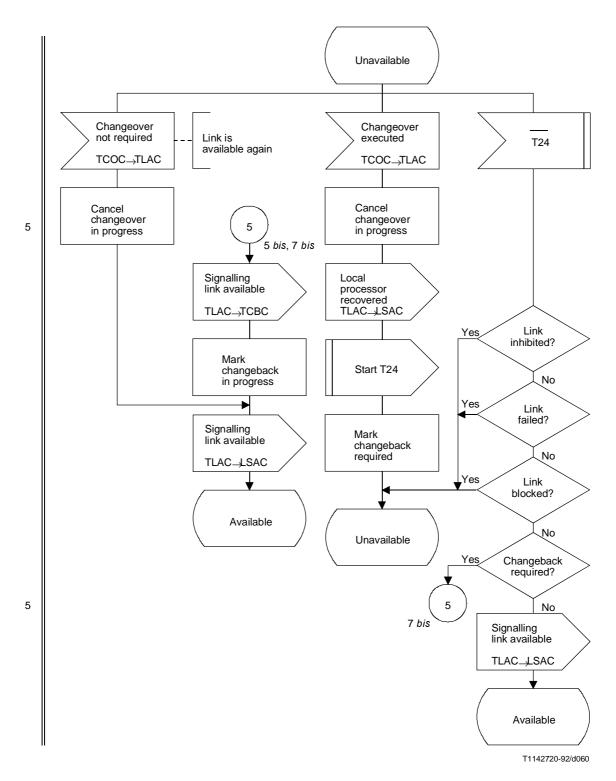
Figure 28/Q.704 (sheet 7 bis of 18) – Signalling traffic management; link availability control (TLAC) (National option)
