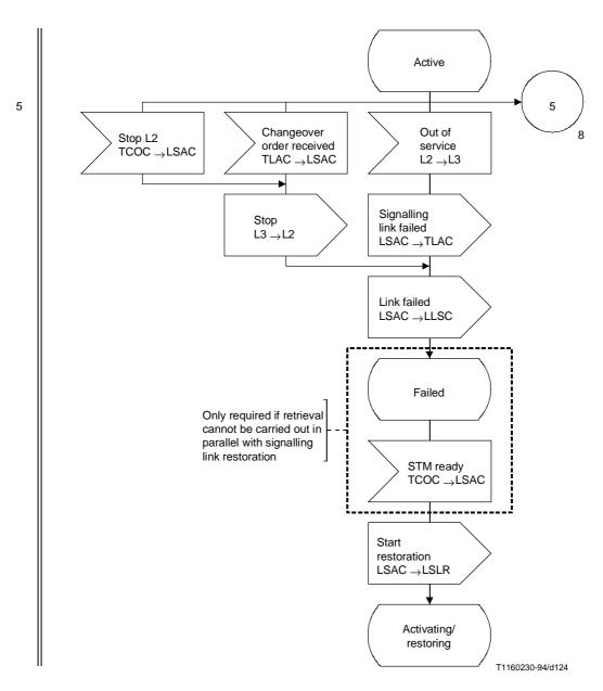
$\label{eq:figure 37/Q.704} Figure \ 37/Q.704 \ (sheet \ 7 \ of \ 10) - Signalling \ link \ management; \\ signalling \ link \ activity \ control \ (LSAC)$
