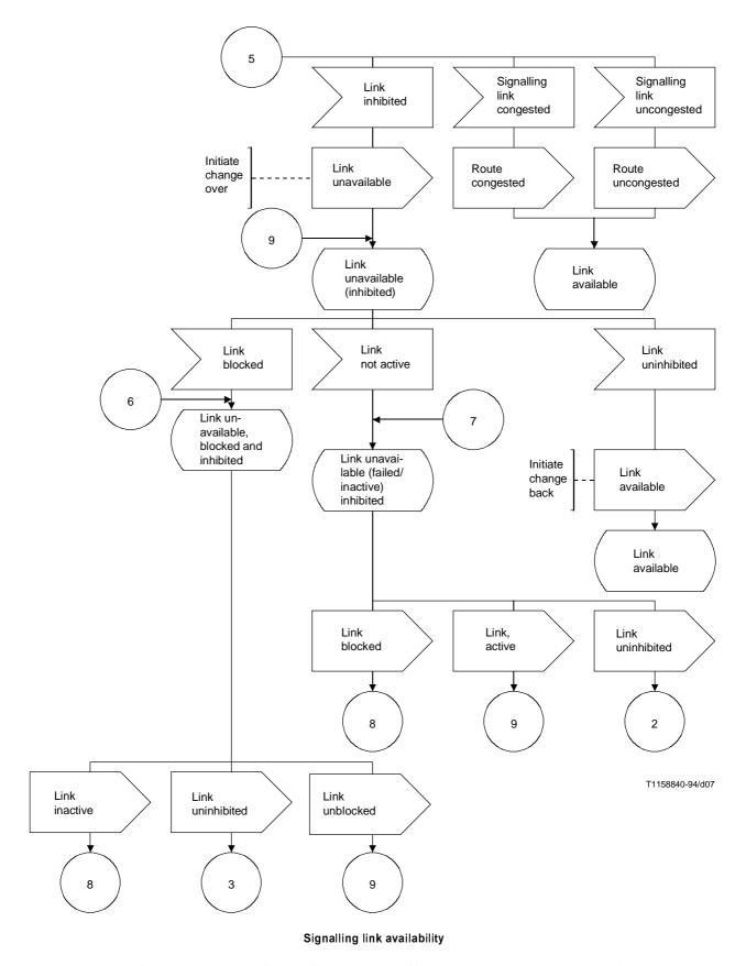
Figure 6/Q.704 (sheet 2 of 4) – Signalling traffic management overview diagram
