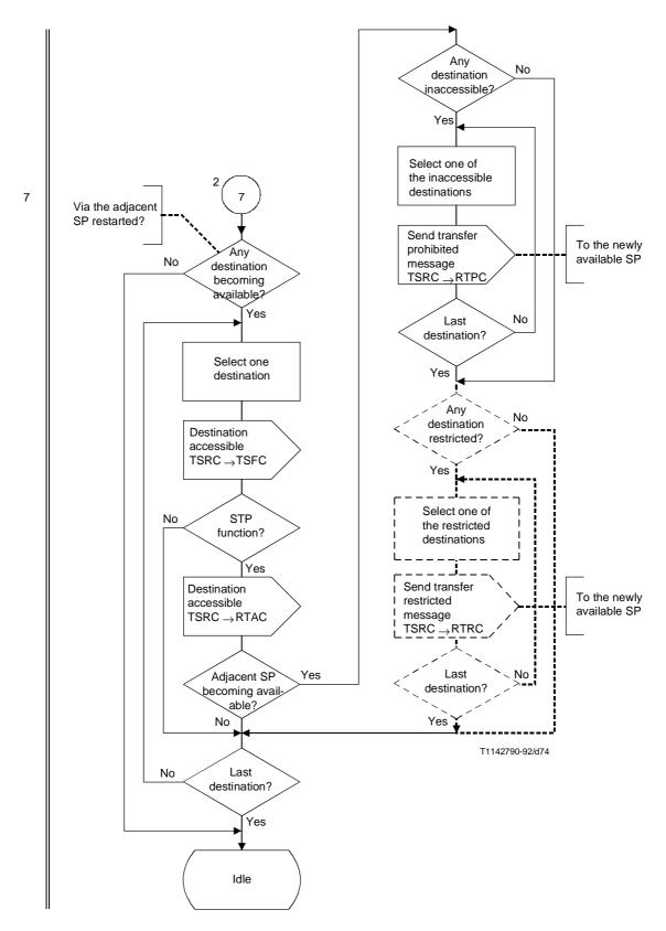
Figure 29/Q.704 (sheet 3 of 21) – Signalling traffic management; signalling routing control (TSRC)
