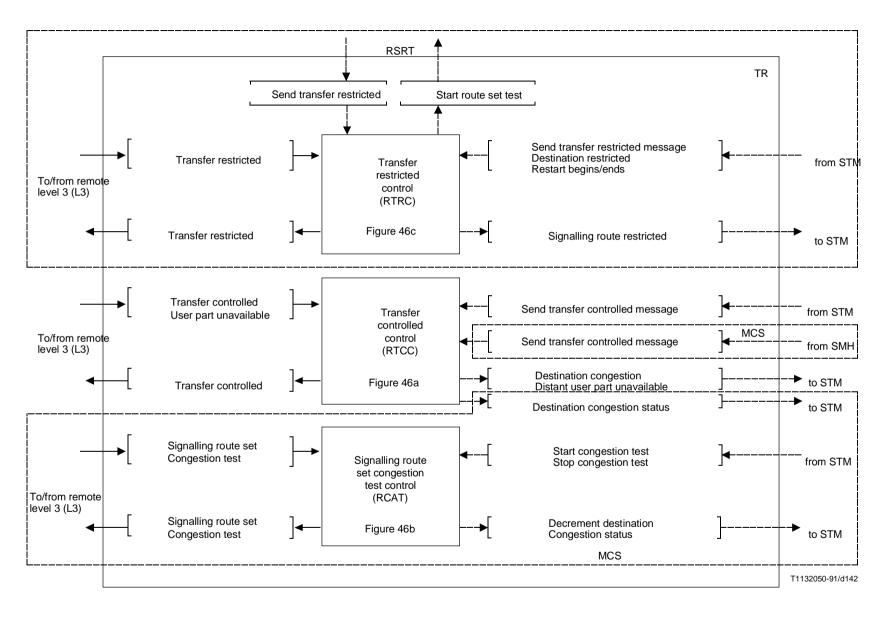
Figure 43/Q.704 (sheet 2 of 2) – Level 3 – Signalling route management (SRM); functional block interactions
