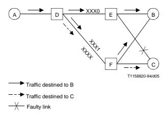
Figure 5/Q.704 – Example of load sharing between link sets
