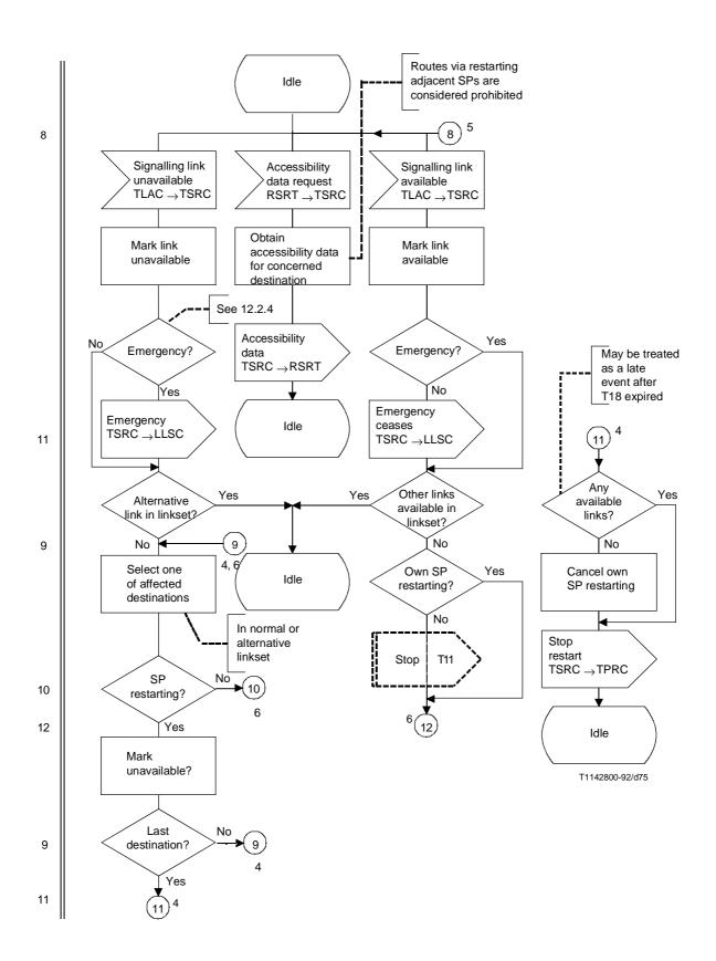
Figure 29/Q.704 (sheet 4 of 21) – Signalling traffic management; signalling routing control (TSRC)
