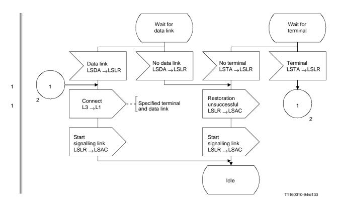
Figure 39/Q.704 (sheet 2 of 2) – Signalling link management; signalling link restoration (LSLR)
