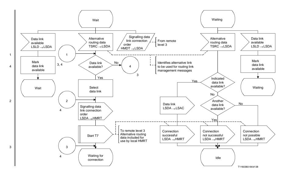
Figure 42/Q.704 (sheet 2 of 4) – Signalling link management; signalling data link allocation (LSDA)
