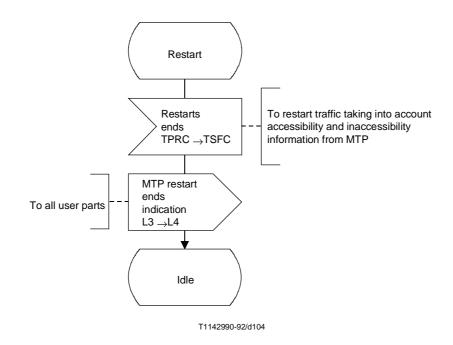
Figure 34a/Q.704 (sheet 2 of 3) – Signalling traffic management; signalling traffic flow control (TSFC)
