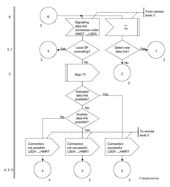
Figure 42/Q.704 (sheet 4 of 4) – Signalling link management; signalling data link allocation (LSDA)
