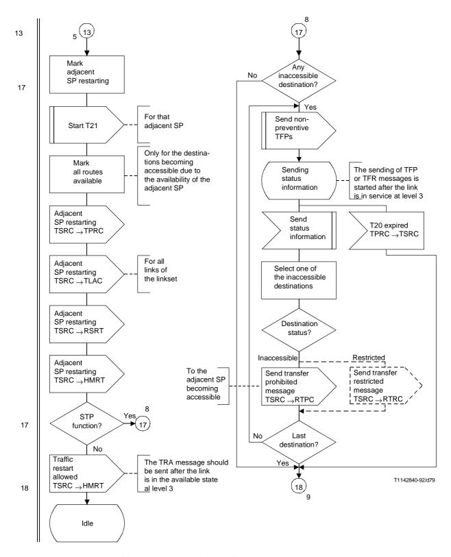
Figure 29/Q.704 (sheet 8 of 21) – Signalling traffic management; signalling routing control (TSRC)
