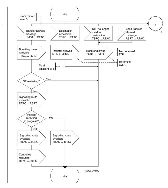
Figure 45/Q.704 (sheet 1 of 2) – Signalling route management; transfer allowed control (RTAC)
