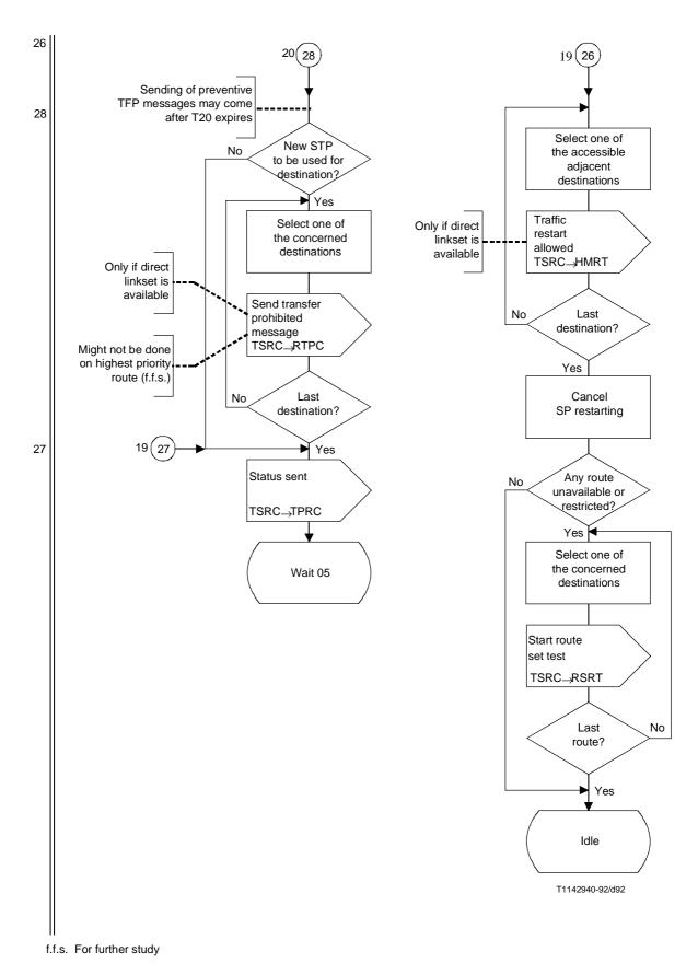
Figure 29/Q.704 (sheet 21 of 21) – Signalling traffic management; signalling routing control (TSRC)
