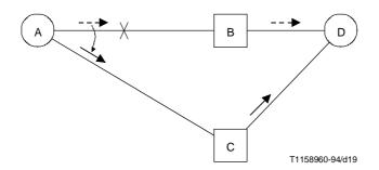
Figure 12/Q.704 – Example of time-controlled diversion procedure
