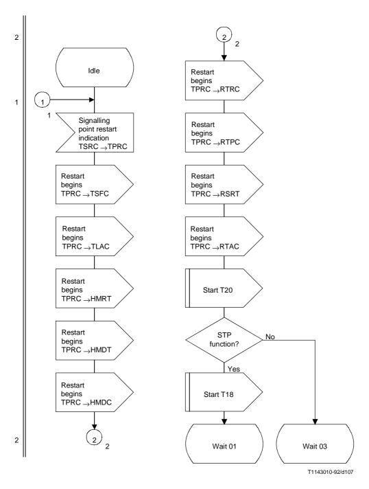
Figure 34b/Q.704 (sheet 2 of 7) – Signalling traffic management; signalling point restart control (TPRC)
