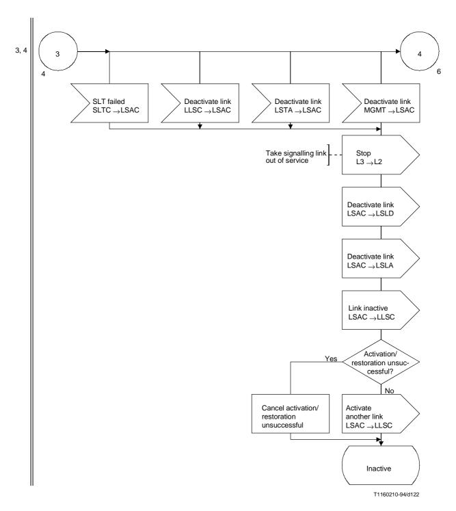
$\label{eq:figure 37/Q.704} Figure \ 37/Q.704 \ (sheet \ 5 \ of \ 10) - Signalling \ link \ management; \\ signalling \ link \ activity \ control \ (LSAC)$
