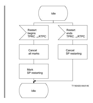
Figure 44/Q.704 (sheet 3 of 3) – Signalling route management; transfer prohibited control (RTPC)
