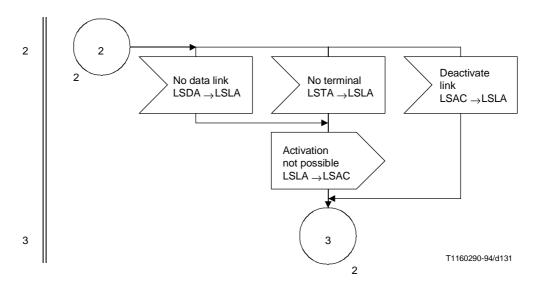
Figure 38/Q.704 (sheet 3 of 3) – Signalling link management; signalling link activation (LSLA)
