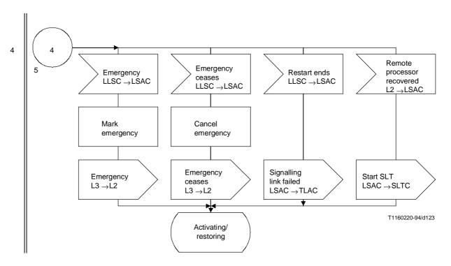
$\label{eq:figure 37/Q.704} Figure \ 37/Q.704 \ (sheet \ 6 \ of \ 10) - Signalling \ link \ management; \\ signalling \ link \ activity \ control \ (LSAC)$
