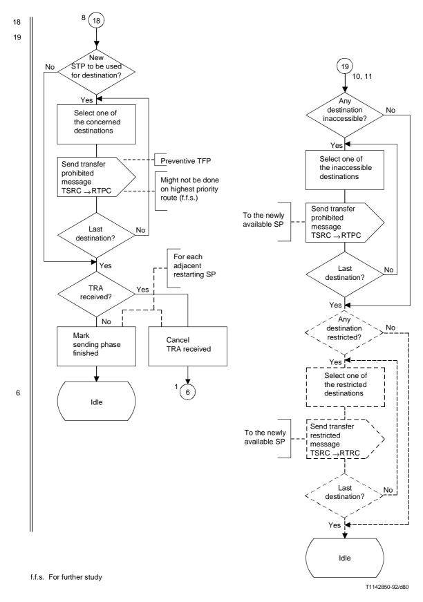
Figure 29/Q.704 (sheet 9 of 21) – Signalling traffic management; signalling routing control (TSRC)
