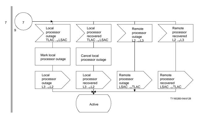
Figure 37/Q.704 (sheet 10 bis of 10) – Signalling link management; signalling link activity control (LSAC) (National option)
