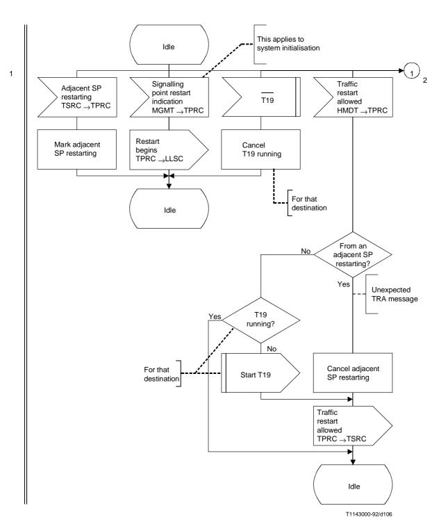
Figure 34b/Q.704 (sheet 1 of 7) – Signalling traffic management; signalling point restart control (TPRC)
