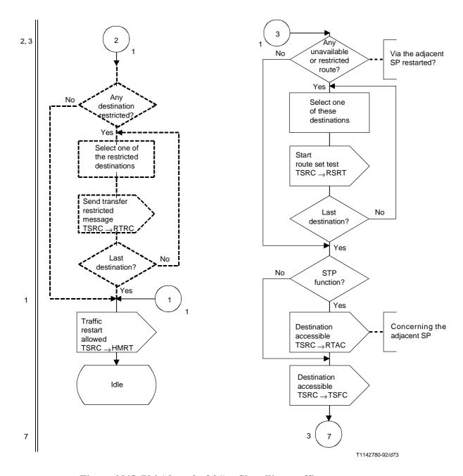
Figure 29/Q.704 (sheet 2 of 21) – Signalling traffic management; signalling routing control (TSRC)
