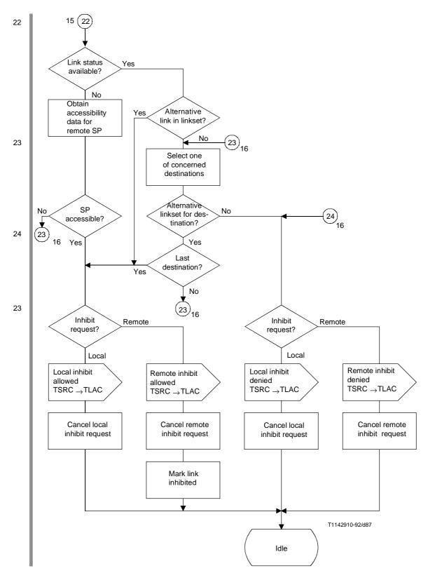
$\label{eq:figure 29/Q.704} Figure \ 29/Q.704 \ (sheet \ 16 \ of \ 21) - Signalling \ traffic \ management; \\ signalling \ routing \ control \ (TSRC)$
