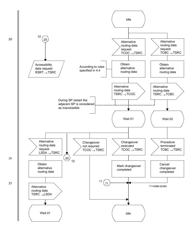
Figure 29/Q.704 (sheet 12 of 21) – Signalling traffic management; signalling routing control (TSRC)
