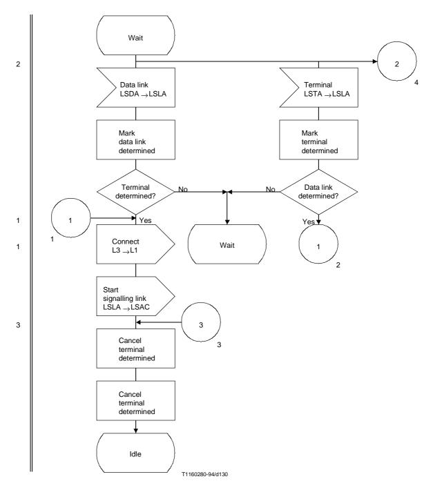
$\label{eq:figure 38/Q.704} Figure \ 38/Q.704 \ (sheet \ 2 \ of \ 3) - Signalling \ link \ management; \\ signalling \ link \ activation \ (LSLA)$
