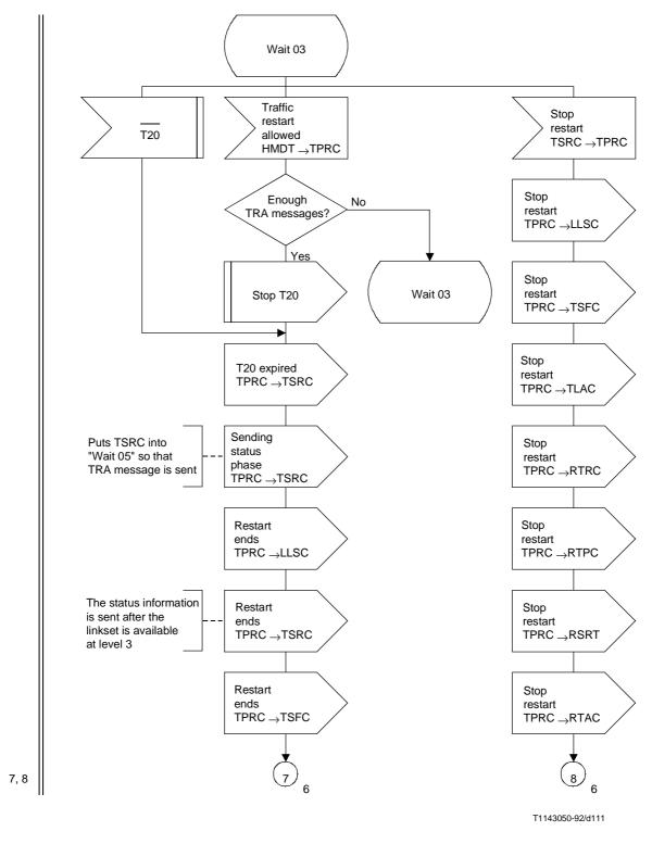
Figure 34b/Q.704 (sheet 6 of 7) – Signalling traffic management; signalling point restart control (TPRC)
