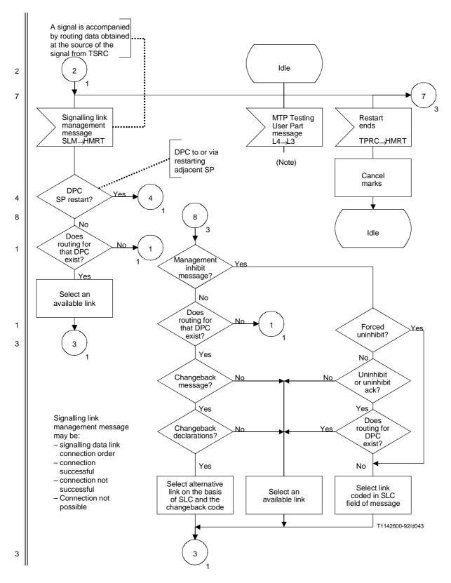
NOTE – Some special routing for MTP Testing User Part may be needed depending on the functions and requirements of such a User Part.
