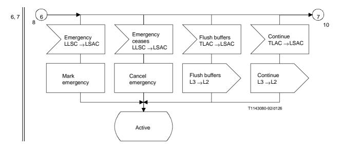
Figure 37/Q.704 (sheet 9 of 10) – Signalling link management; signalling link activity control (LSAC)
