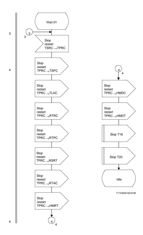
Figure 34b/Q.704 (sheet 4 of 7) – Signalling traffic management; signalling point restart control (TPRC)
