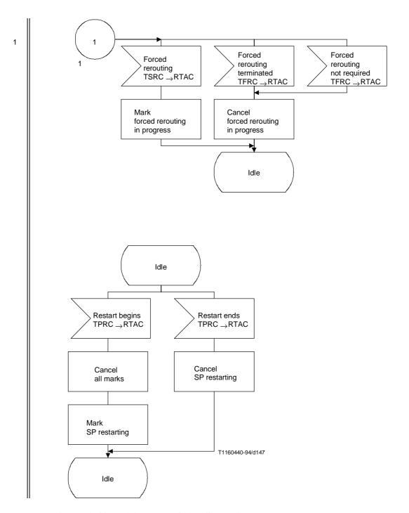
Figure 45/Q.704 (sheet 2 of 2) – Signalling route management; transfer allowed control (RTAC)
