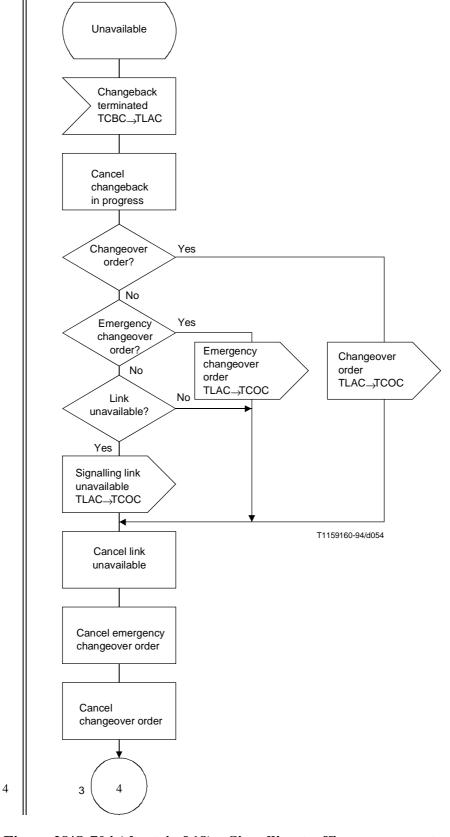
Figure 28/Q.704 (sheet 4 of 18) – Signalling traffic management; link availability control (TLAC)
