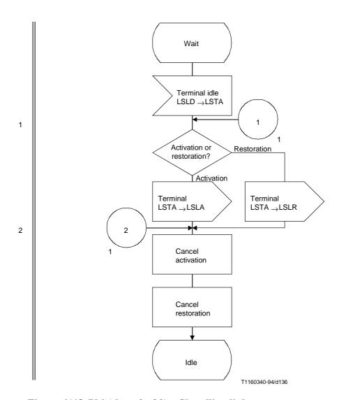
Figure 41/Q.704 (sheet 2 of 2) – Signalling link management; signalling terminal allocation (LSTA)
