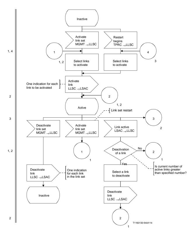
Figure 36/Q.704 (sheet 1 of 3) – Signalling link management; link set control (LLSC)
