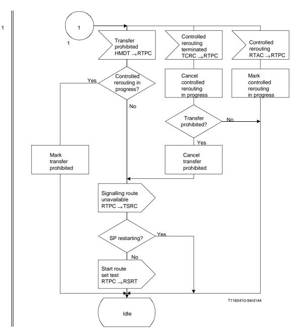
Figure 44/Q.704 (sheet 2 of 3) – Signalling route management; transfer prohibited control (RTPC)
