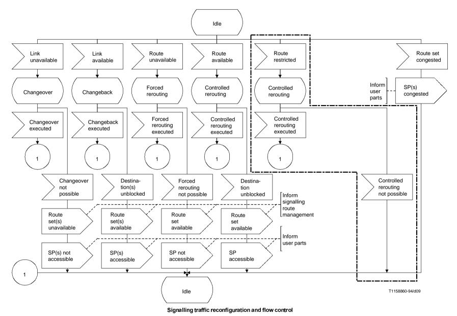
Figure 6/Q.704 (sheet 4 of 4) – Signalling traffic management overview diagram
