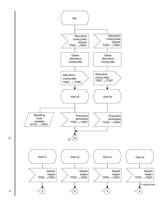
Figure 29/Q.704 (sheet 13 of 21) – Signalling traffic management; signalling routing control (TSRC)
