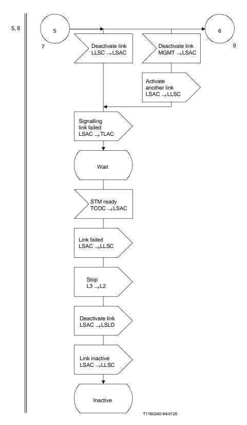
$\label{eq:figure 37/Q.704} Figure \ 37/Q.704 \ (sheet \ 8 \ of \ 10) - Signalling \ link \ management; \\ signalling \ link \ activity \ control \ (LSAC)$
