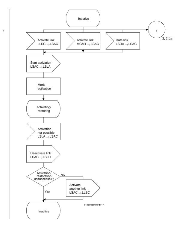
$\label{eq:figure 37/Q.704} Figure \ 37/Q.704 \ (sheet \ 1 \ of \ 10) - Signalling \ link \ management; \\ signalling \ link \ activity \ control \ (LSAC)$
