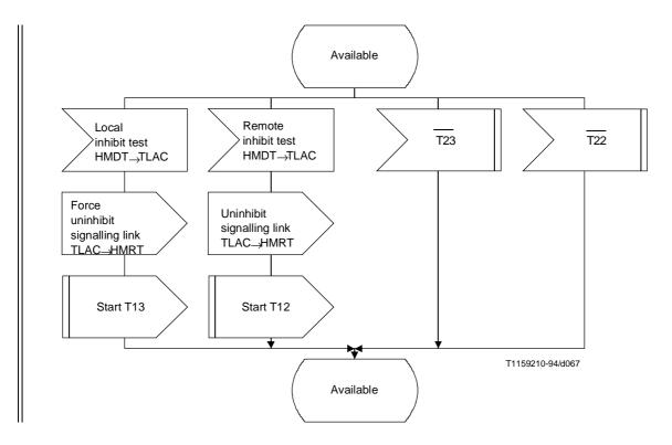
Figure 28/Q.704 (sheet 14 of 18) – Signalling traffic management; link availability control (TLAC)
