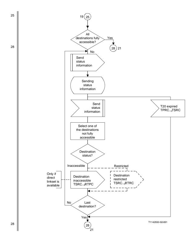
Figure 29/Q.704 (sheet 20 of 21) – Signalling traffic management; signalling routing control (TSRC)
