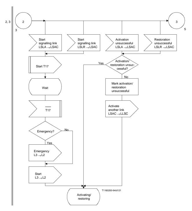
$\label{eq:figure 37/Q.704} Figure \ 37/Q.704 \ (sheet \ 4 \ of \ 10) - Signalling \ link \ management; \\ signalling \ link \ activity \ control \ (LSAC)$
