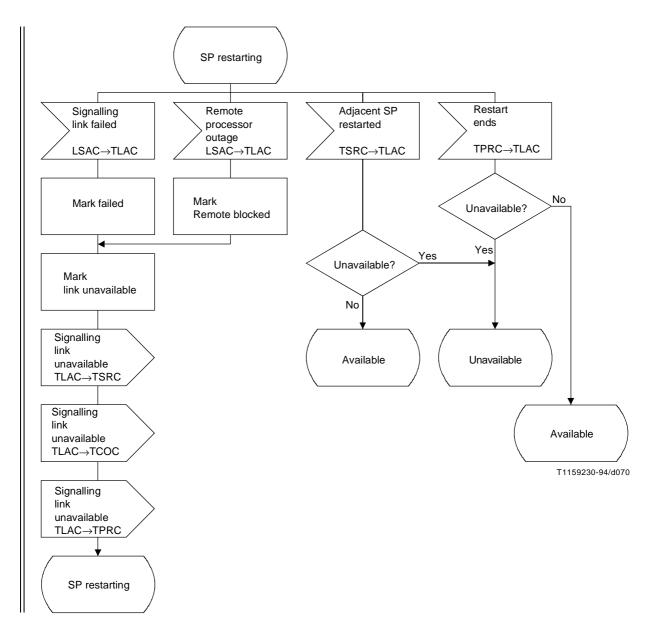
Figure 28/Q.704 (sheet 17 of 18) – Signalling traffic management; link availability control (TLAC)
