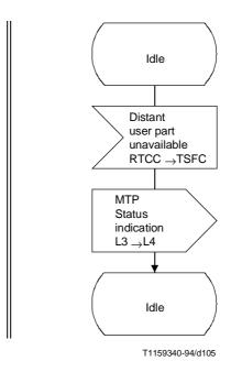
$\label{eq:signal-signal} Figure~34a/Q.704~(sheet~3~of~3)-Signalling~traffic~management;\\ signalling~traffic~flow~control~(TSFC)$
