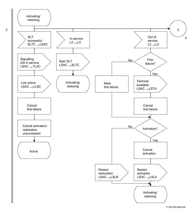
Figure 37/Q.704 (sheet 3 of 10) – Signalling link management; signalling link activity control (LSAC)
