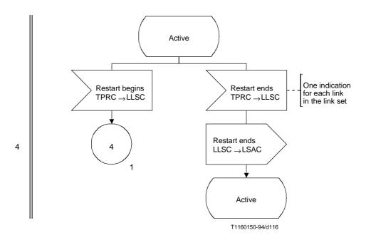
Figure 36/Q.704 (sheet 3 of 3) – Signalling link management; link set control (LLSC)
