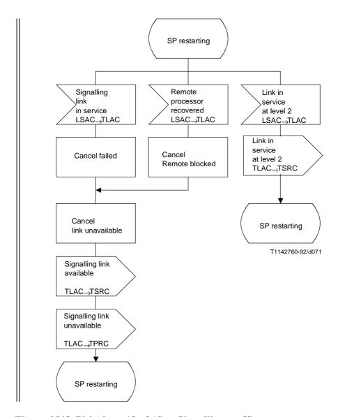
Figure 28/Q.704 (sheet 18 of 18) – Signalling traffic management; link availability control (TLAC)
