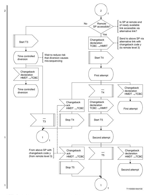
$\label{eq:NOTE-For simplicity} \mbox{NOTE} - \mbox{For simplicity, changeback from only one alternative link is shown.}$
