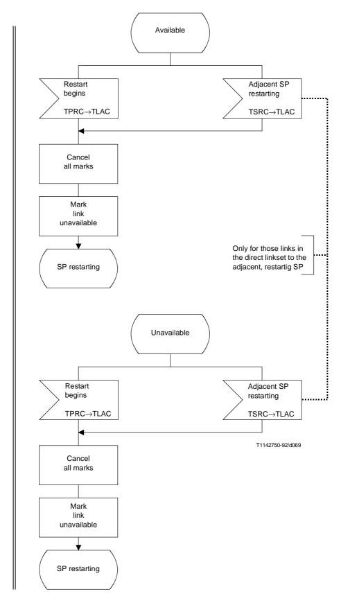
Figure 28/Q.704 (sheet 16 of 18) – Signalling traffic management; link availability control (TLAC)
