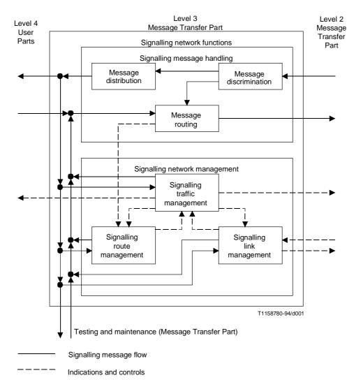
Figure 1/Q.704 – Signalling network functions
