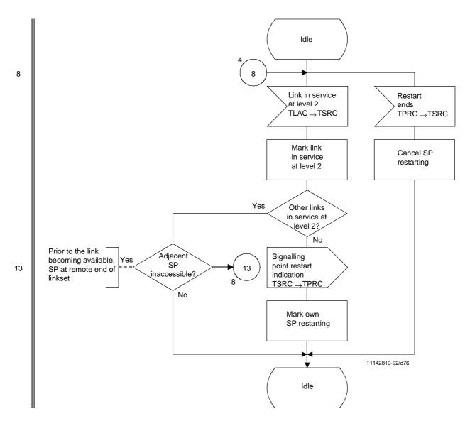
Figure 29/Q.704 (sheet 5 of 21) – Signalling traffic management; signalling routing control (TSRC)
