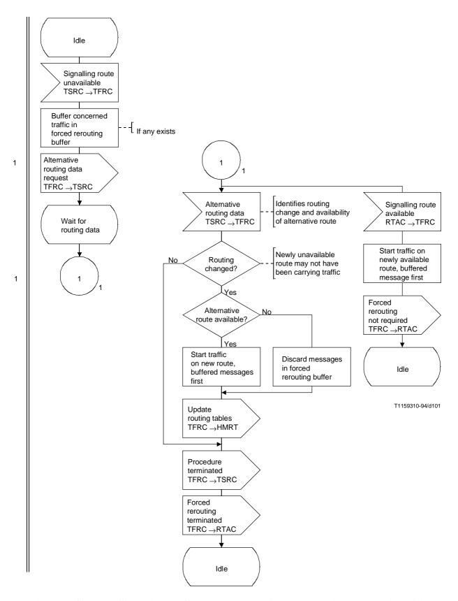
Figure 32/Q.704 – Signalling traffic management; forced rerouting control (TFRC)
