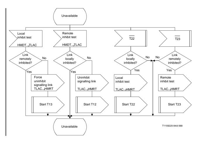
Figure 28/Q.704 (sheet 15 of 18) – Signalling traffic management; link availability control (TLAC)
