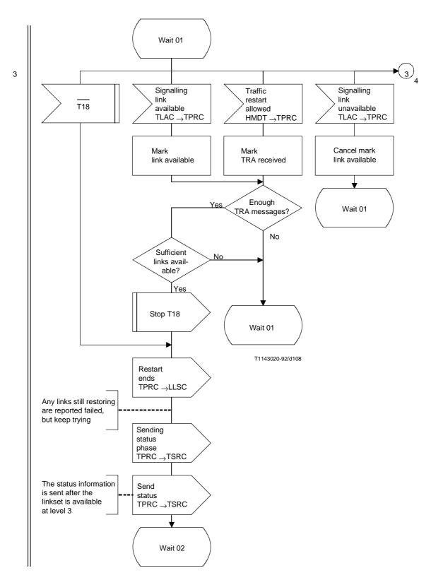
Figure 34b/Q.704 (sheet 3 of 7) – Signalling traffic management; signalling point restart control (TPRC)
