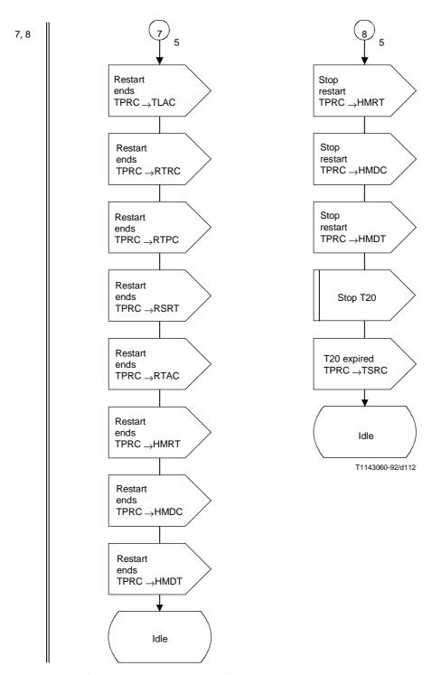
Figure 34b/Q.704 (sheet 7 of 7) – Signalling traffic management; signalling point restart control (TPRC)
