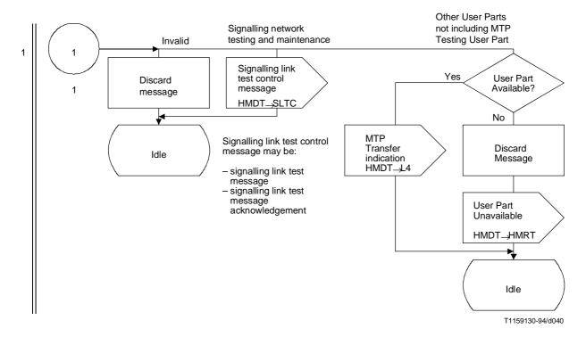
Figure 25/Q.704 (sheet 2 of 3) – Signalling message handling; message distribution (HMDT)
