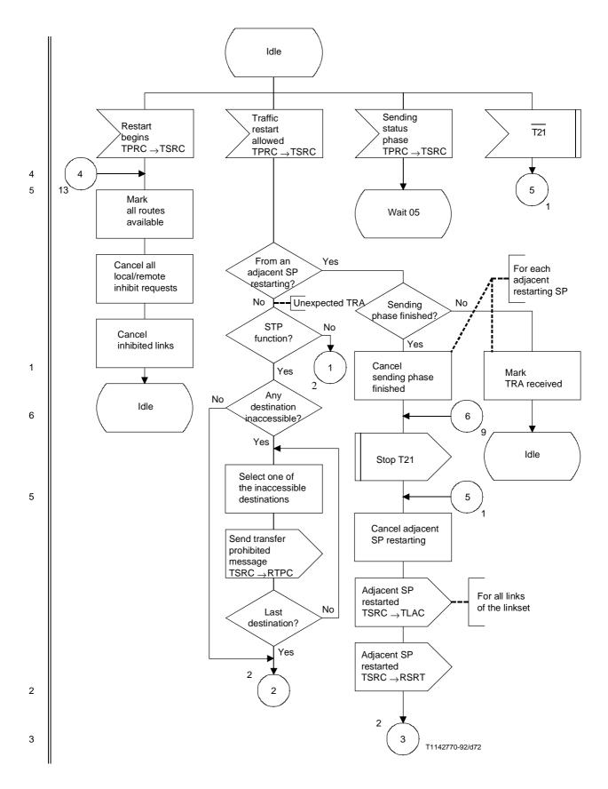
Figure 29/Q.704 (sheet 1 of 21) – Signalling traffic management; signalling routing control (TSRC)
