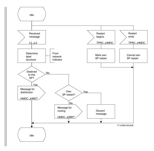
Figure 24/Q.704 – Signalling message handling; message discrimination (HMDC)
