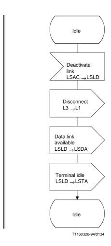
Figure 40/Q.704 – Signalling link management; signalling link deactivation (LSLD)
