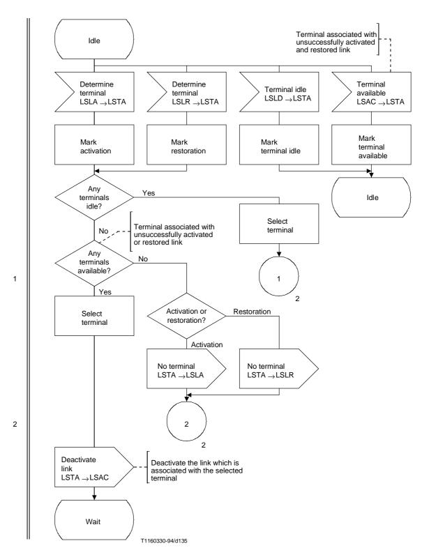
Figure 41/Q.704 (sheet 1 of 2) – Signalling link management; signalling terminal allocation (LSTA)
