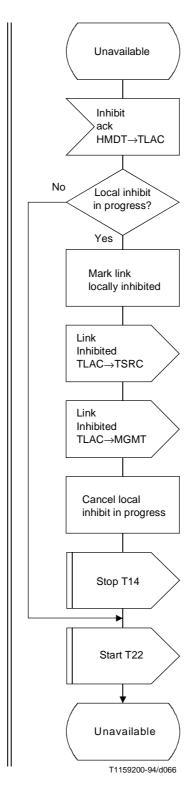
$\label{eq:figure 28/Q.704} Figure \ 28/Q.704 \ (sheet \ 13 \ of \ 18) - Signalling \ traffic \ management; \\ link \ availability \ control \ (TLAC)$
