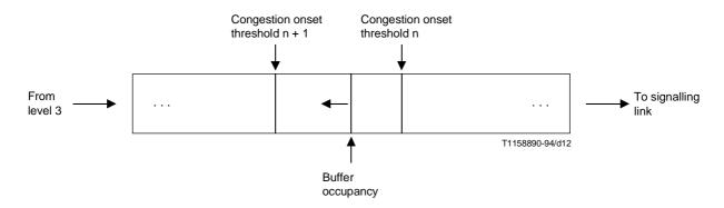
Figure 8a/Q.704 – Signalling link congestion status = n (congestion onset)
