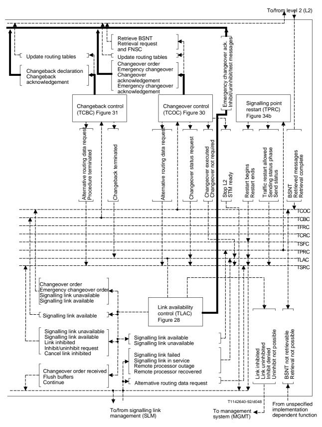
NOTE - Abbreviation message names have been used in this diagram (i.e. origin-destination codes are omitted).
