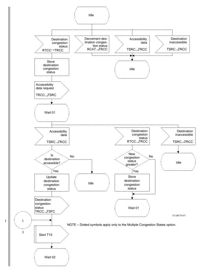
Figure 29a/Q.704 (sheet 1 of 3) – Signalling traffic management; signalling route set congestion control (TRCC)
