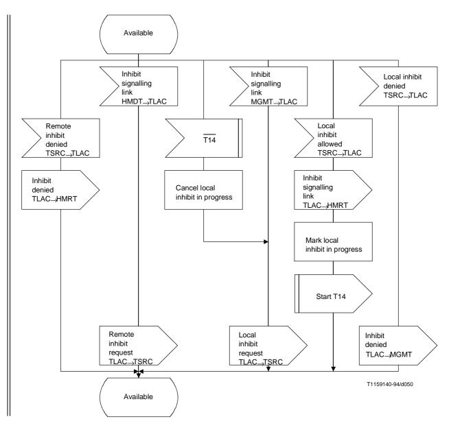
Figure 28/Q.704 (sheet 1 of 18) – Signalling traffic management; link availability control (TLAC)
