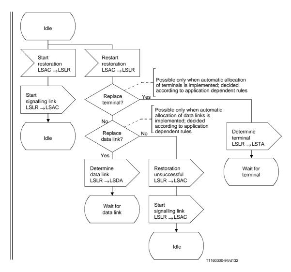
Figure 39/Q.704 (sheet 1 of 2) – Signalling link management; signalling link restoration (LSLR)
