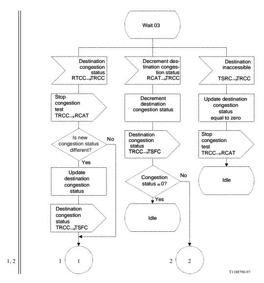
Figure 29a/Q.704 (sheet 3 of 3) – Signalling traffic management; signalling route set congestion control (TRCC)
