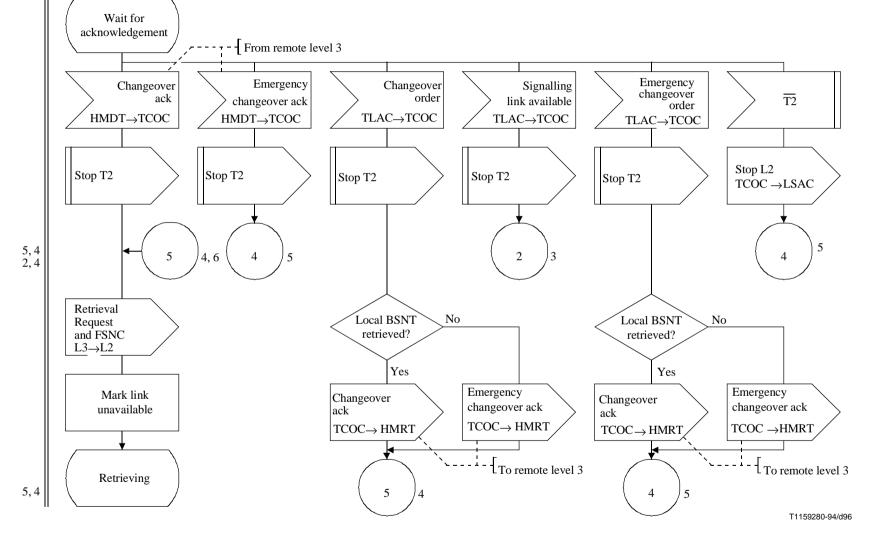
Figure 30/Q.704 (sheet 4 of 6) – Signalling traffic management; changeover control (TCOC)
