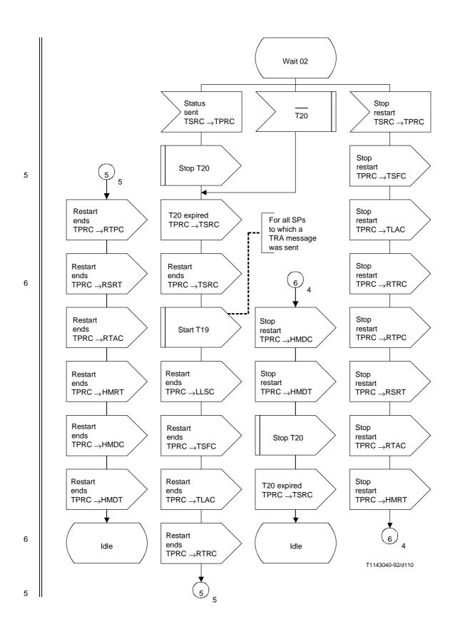
Figure 34b/Q.704 (sheet 5 of 7) – Signalling traffic management; signalling point restart control (TPRC)
