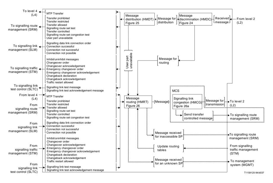
Figure 23/Q.704 – Level 3 – Signalling message handling (SMH); functional block interactions
