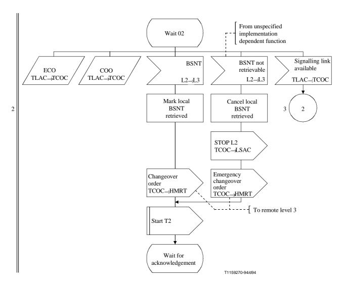
Figure 30/Q.704 (sheet 2 of 6) – Signalling traffic management; changeover control (TCOC)
