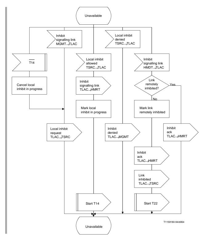
Figure 28/Q.704 (sheet 11 of 18) – Signalling traffic management; link availability control (TLAC)
