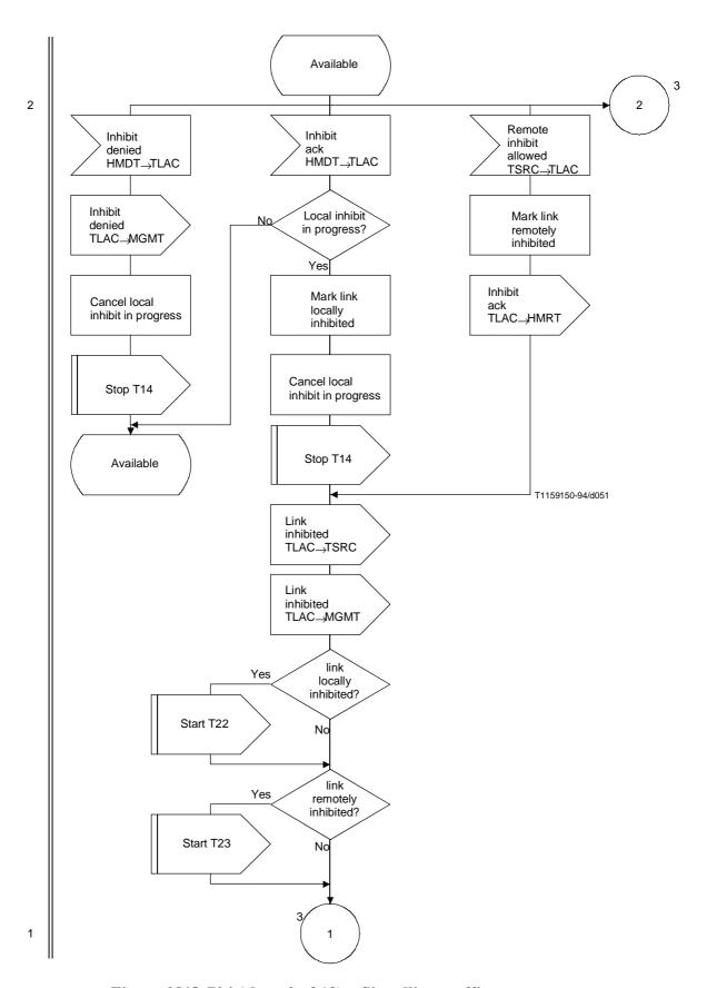
$\label{eq:signal-signal} Figure~28/Q.704~(sheet~2~of~18)-Signalling~traffic~management;\\ link~availability~control~(TLAC)$
