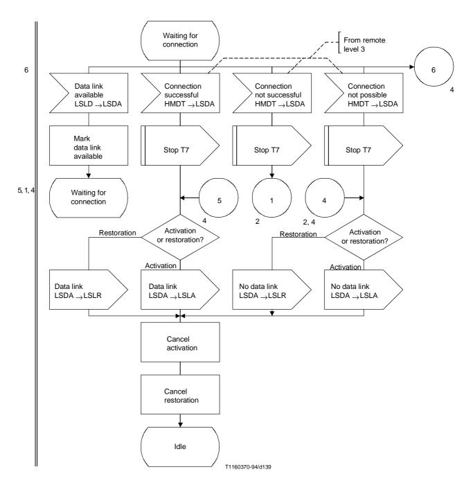
Figure 42/Q.704 (sheet 3 of 4) – Signalling link management; signalling data link allocation (LSDA)
