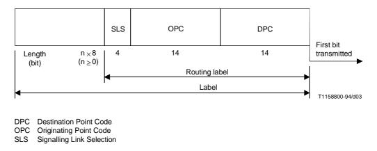
Figure 3/Q.704 – Routing label structure
