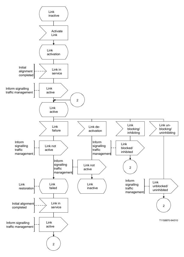
Figure 7/Q.704 – Signalling link management overview diagram
