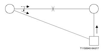
Figure 10/Q.704 – Example of changeover to a signalling route passing through the remote signalling point
