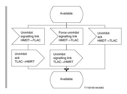
Figure 28/Q.704 (sheet 12 of 18) – Signalling traffic management; link availability control (TLAC)
