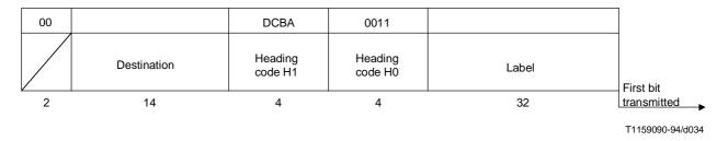
Figure 22b/Q.704 - Transfer-controlled message
