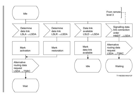
$\label{eq:figure 42/Q.704} Figure \ 42/Q.704 \ (sheet \ 1 \ of \ 4) - Signalling \ link \ management; \\ signalling \ data \ link \ allocation \ (LSDA)$
