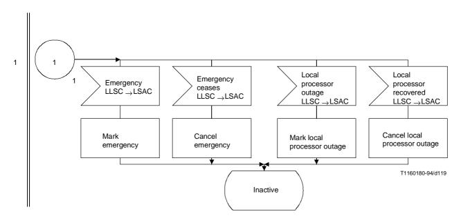
Figure 37/Q.704 (sheet 2 bis of 10) – Signalling link management; signalling link activity control (LSAC)
