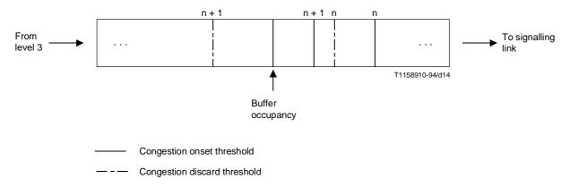
Figure 8c/Q.704 – Signalling link congestion status = n
