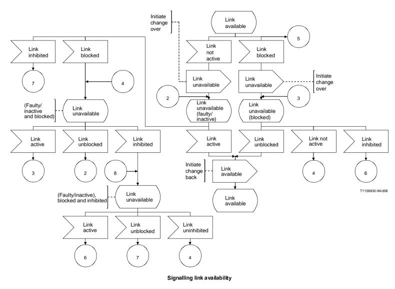
NOTE - Link not active signal represents both link failure and link deactivation. Link active signal represents both link restoration and link activation.
