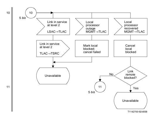
Figure 28/Q.704 (sheet 6 bis of 18) – Signalling traffic management; link availability control (TLAC) (National option)
