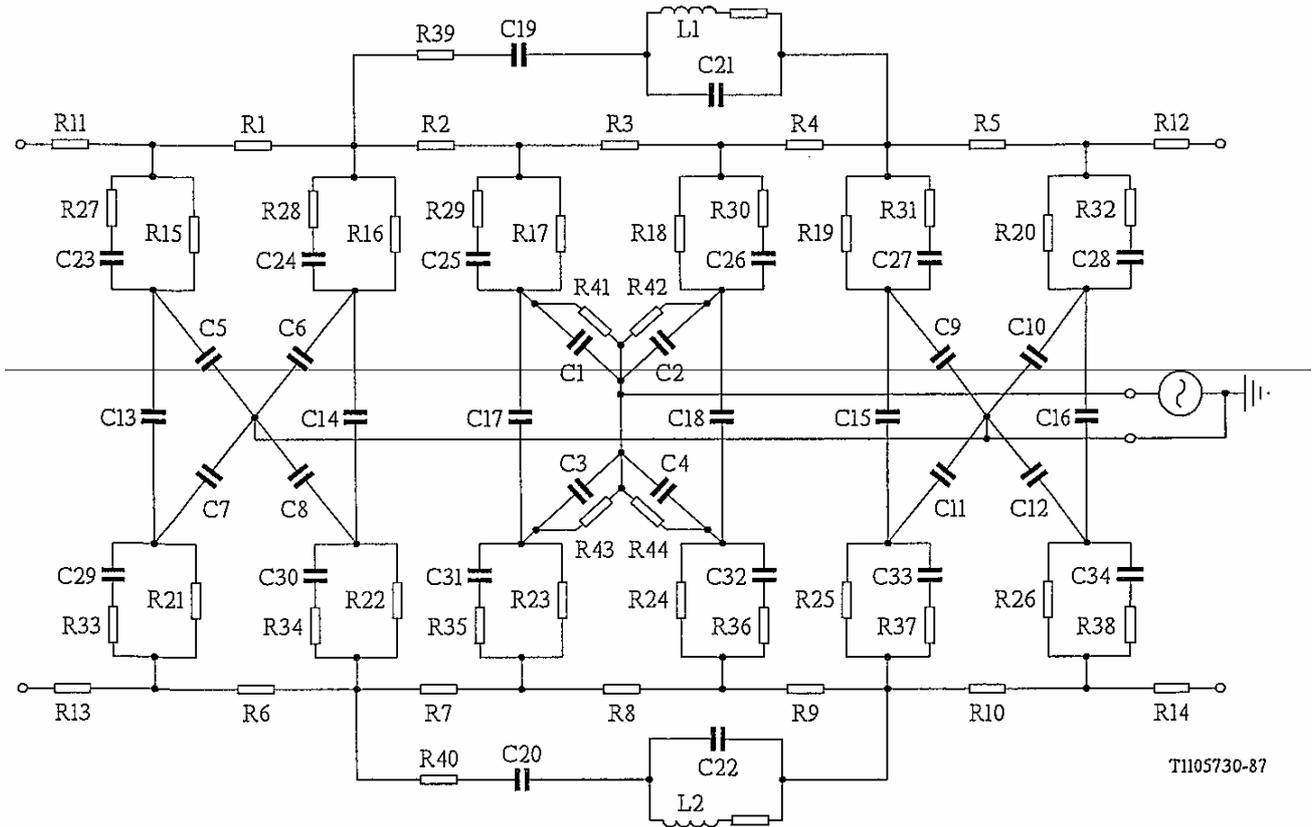
Note -- The component values given in Table A-1/Q.552 are applicable to 4 km of 0.4 mm cable with a mutual capacitance of 47 nF/km and a capacitance to earth of 15 nF/km.
