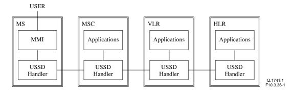
Figure 10-3/Q.1741.1 – Handling of USSD
