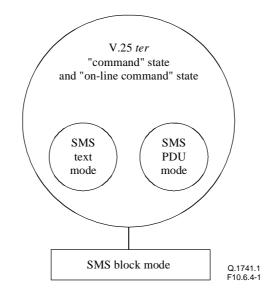
Figure 10-4/Q.1741.1 – Block, text and PDU modes
