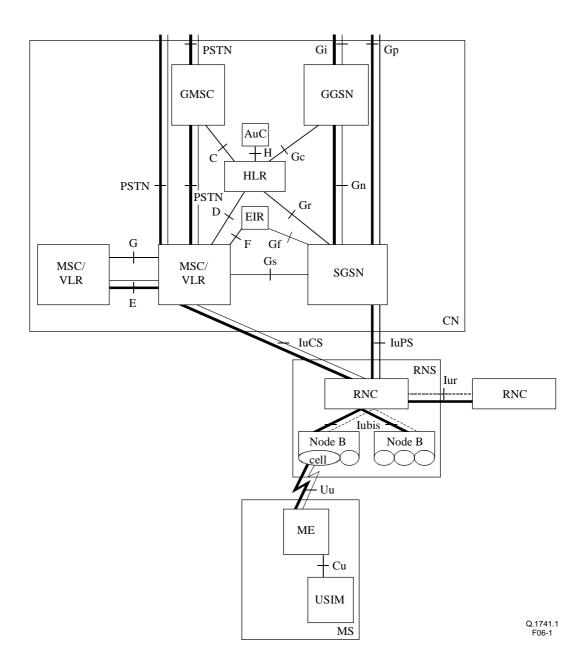
Bold linesInterfaces supporting user trafficDashed linesInterfaces supporting signalling
