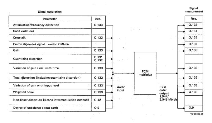
Note – Measurements performed via the digital interface of a primary PCM multiplexer are generally applicable also to transmultiplexers conforming to Recommendations G.793 [1] and G.794 [2]. Where relevant, a suitable analogue test signal generator is assumed.
