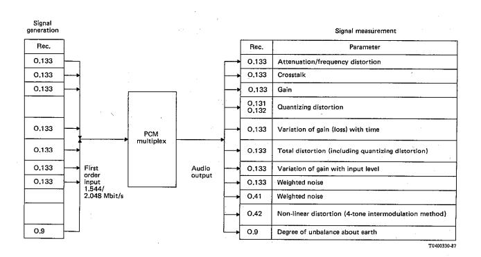
Note – Measurements performed via the digital interface of a primary PCM multiplexer are generally applicable also to transmultiplexers conforming to Recommendations G.793 [1] and G.794 [2]. Where relevant, a suitable analogue test signal measurement capability is assumed.
