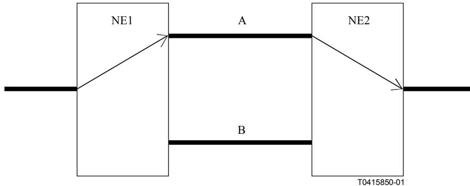
Figure 10/M.3100 – Unidirectional cross-connection
