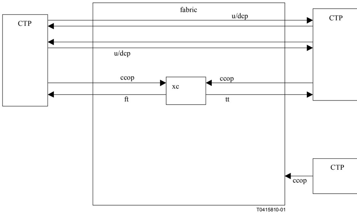
**Figure 6/M.3100 – Initial configuration (point-to-point bidirectional)**
