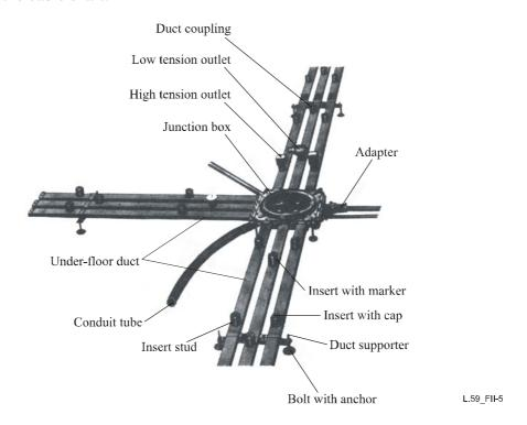
Figure II.5/L.59 – Outline of under-floor duct system
