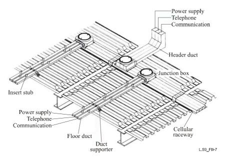
Figure II.7/L.59 – Outline of cellular raceway system
