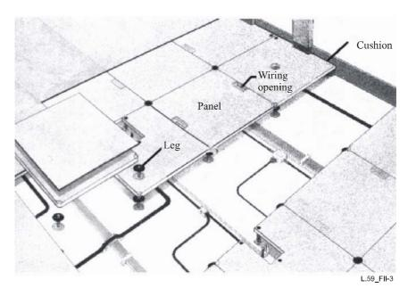
Figure II.3/L.59 – Example of simplified access floor system (Panel-leg separate type)
