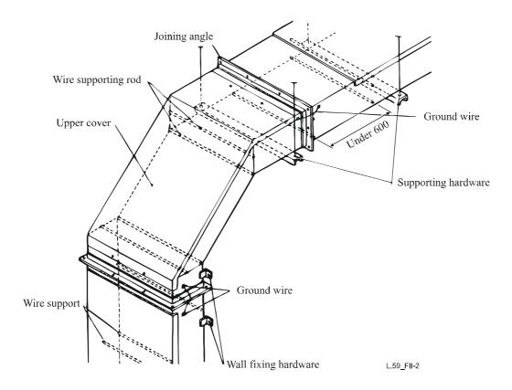
Figure II.2/L.59 – Metal duct system
