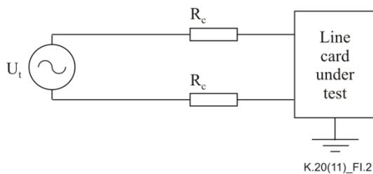
Special test protectors may be used in front of the line card under test if the test is extended to higher voltages.
