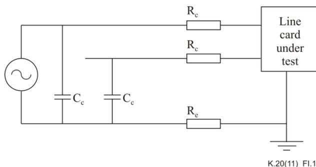
Coupling resistors,  $R_c$ , represent the line resistances; capacitances,  $C_c$ , represent the line capacitances to earth and  $R_e$  represents the earthing resistance of the overvoltage protectors at the subscriber end of the line.
