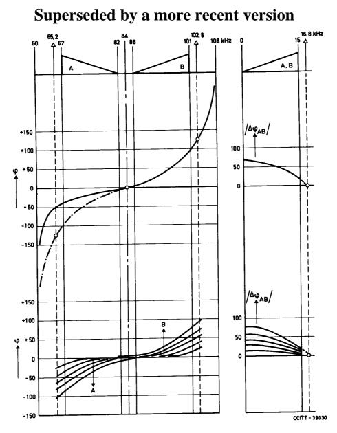
Top: Example of phase symmetry distortion. Ideal skew-symmetric phase characteristic shown. Bottom: Fan-shaped characteristics of the phase-symmetry equalizers.
