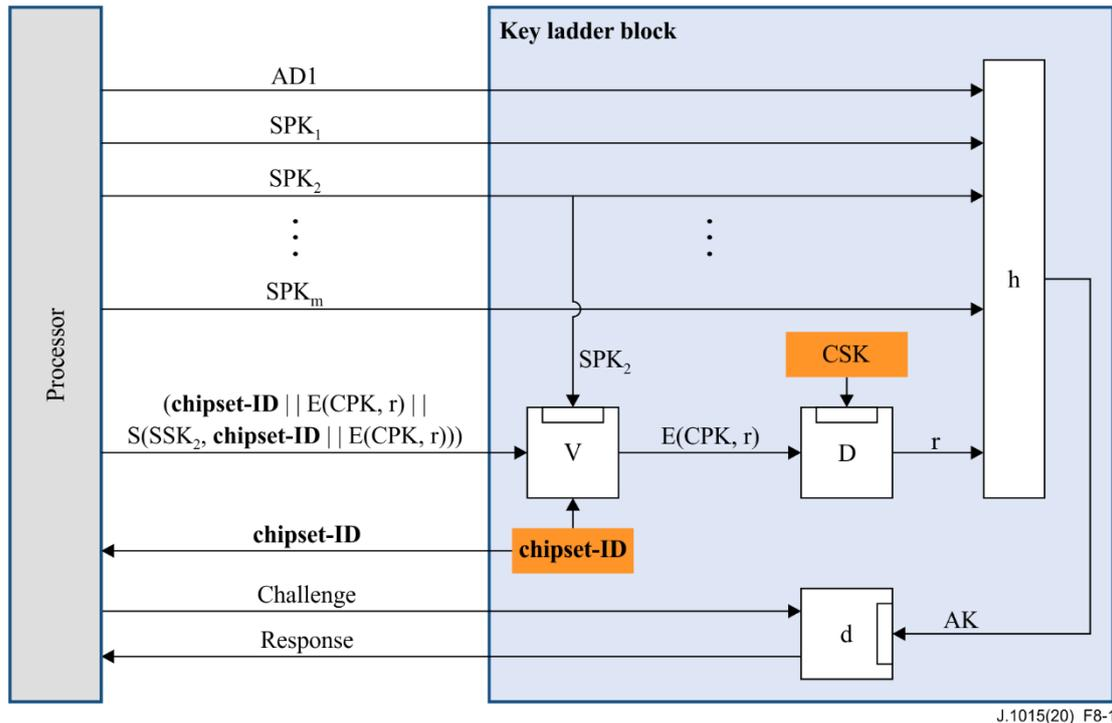
Figure 8-1 – Authentication mechanism
