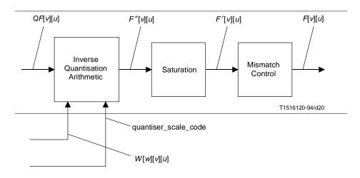
**Figure 7-4** – **Inverse quantisation process**
