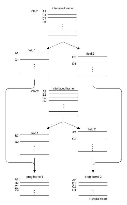
Figure D.4 – Two-interlace to progressive conversion
