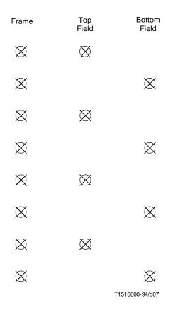
Figure 6-6 – Vertical positions of samples with 4:2:2 and 4:4:4 data
