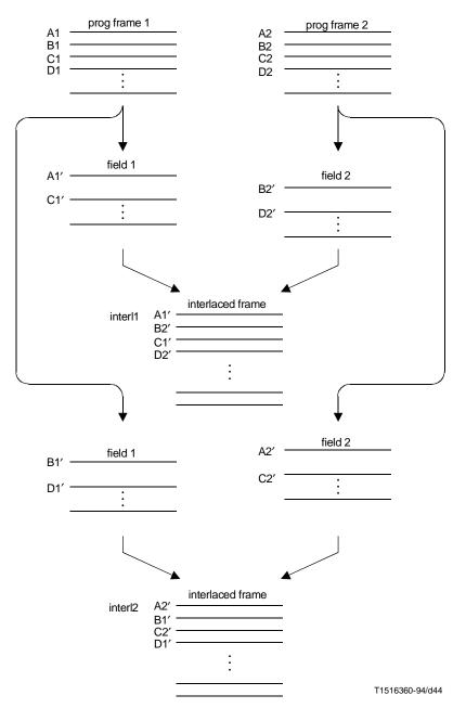
Figure D.3 – Progressive to two-interlace conversion
