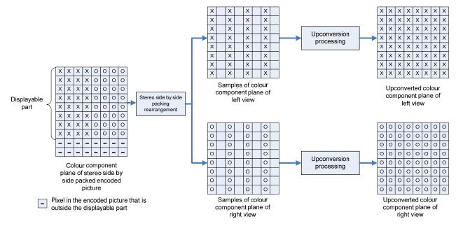
Figure L.1 – Rearrangement and hypothetical upconversion of "stereo side by side" arrangement views to convert to the full resolution of the displayable part of the encoded picture
