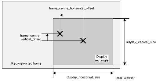
Figure 6-16 – Frame centre offset parameters
