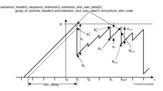
Figure C.1 – VBV Buffer Occupancy – Constant bit-rate operation
