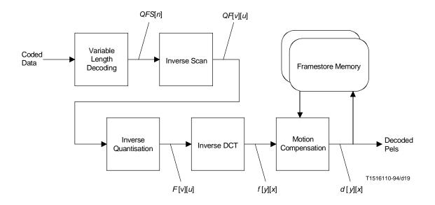
Figure 7-1 – Simplified Video Decoding Process
