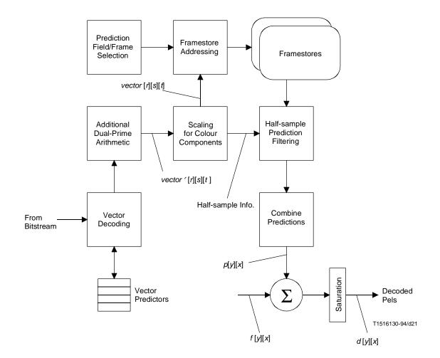
Figure 7-5 – Simplified motion compensation process
