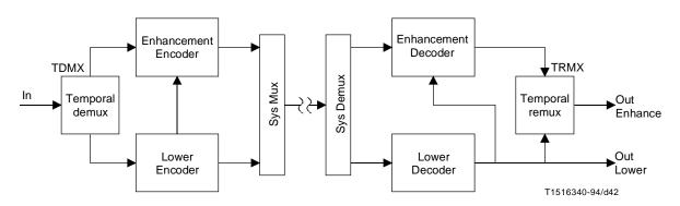
Figure D.1 – A two-layer codec structure for temporal scalability
