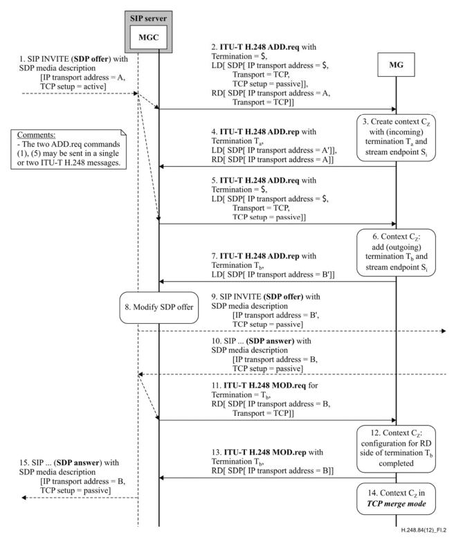
Figure I.2 – ITU-T H.248 signalling for TCP mode assignment – Here: TCP merge mode
