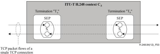
NOTE - A TCP connection is inherently bidirectional (opposed to, e.g., UDP) due to the connection-oriented property.
