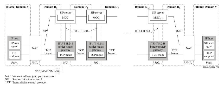
Figure 2 – Reference model for the example of TCP bearer and SIP signalling path with multiple, k-1 MGs in the end-to-end TCP path
