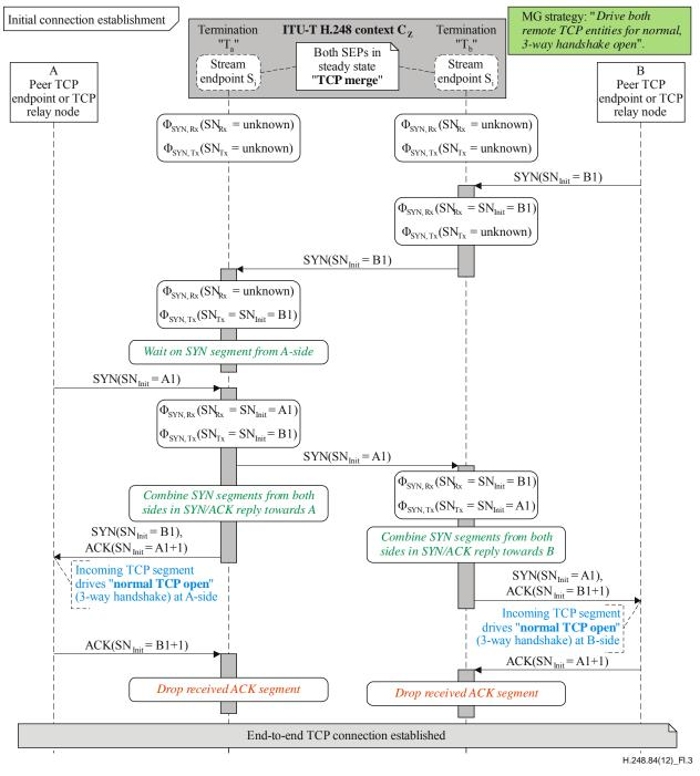
Figure I.3 – Successful resolution of a simultaneous TCP open situation by an ITU-T H.248 MG in TCP merge mode (MG strategy: "Drive both remote TCP entities for normal, 3-way handshake open") Some notes to the signalling flow (Figure I.3):
