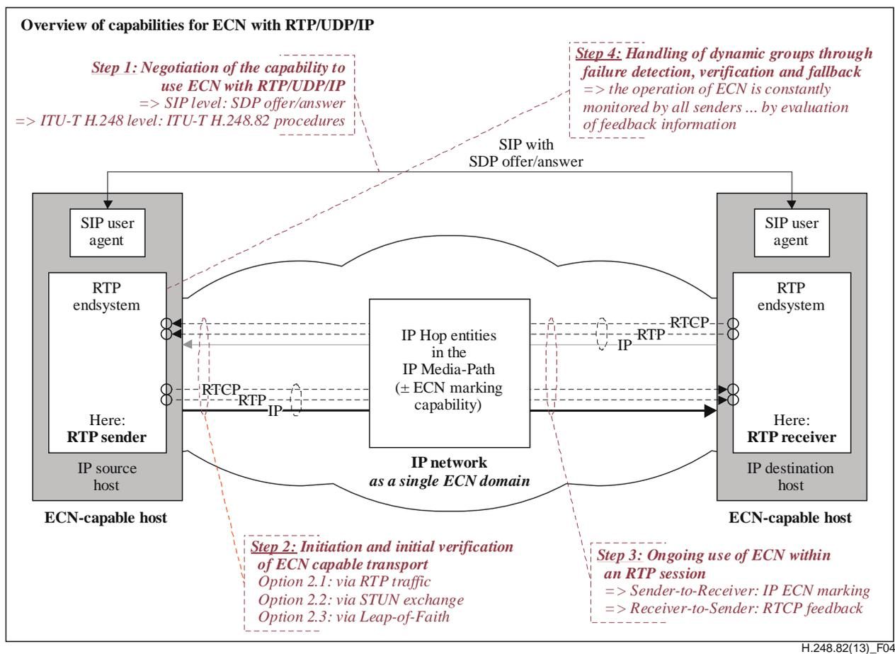
**Figure 4 – Procedures for use of ECN with RTP-over-UDP traffic**
