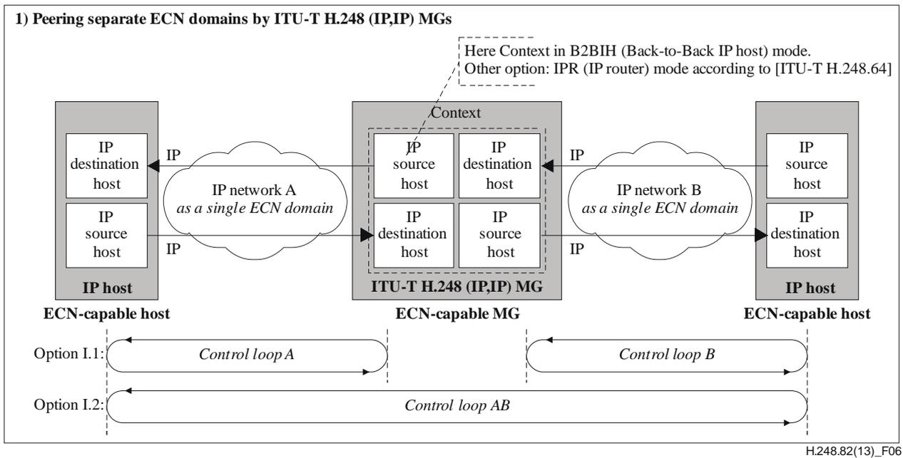
NOTE – The IP topologies are basically associated with the ITU-T H.248 Stream level. The figure above illustrates an example on Context level (referred to the IP topology models according to clause 3.2.1 (B2BIH) and clause 6.5.1 (IP router) of [ITU-T H.248.64]).
