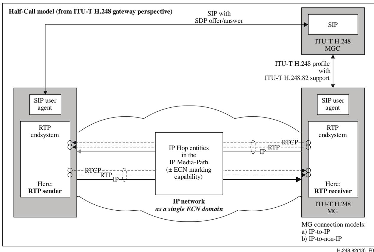
**Figure 5 – Control plane example with ITU-T H.248 network elements at the edge of an ECN domain**
