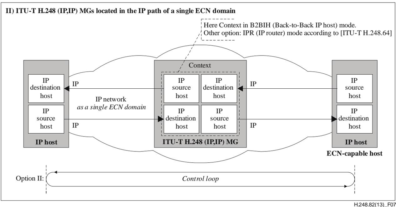
**Figure 7 – ITU-T H.248 (IP,IP) MGs located in the IP path of a single ECN domain**
