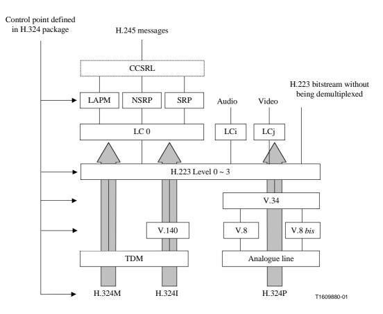
Figure M4-1/H.248 – Control point defined in H.324 package
