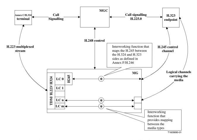
Figure M4-2/H.248 – Resource control at the MG (without fastStart/H.245 tunnelling)
