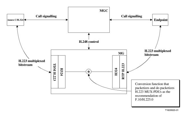
Figure M4-5/H.248 – Configuration for IP tunnelling of Annex C/H.324 bitstream
