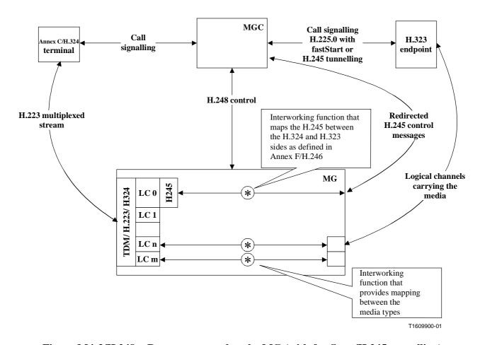
Figure M4-3/H.248 – Resource control at the MG (with fastStart/H.245 tunnelling)
