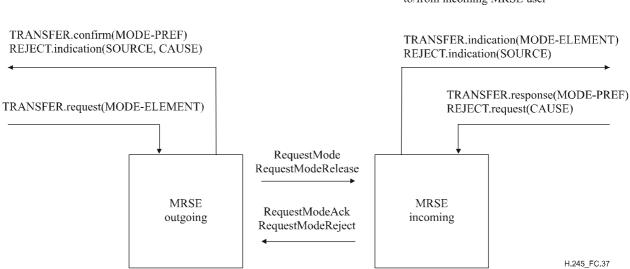
Figure C.37/H.245 – Primitives and messages in the Mode Request Signalling Entity
