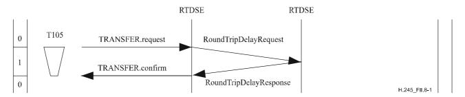
Figure II.8-1/H.245 – Round-trip delay determination procedure
