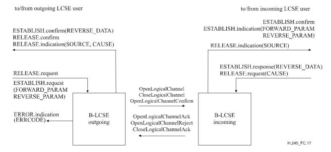
Figure C.17/H.245 – Primitives and messages in the bidirectional Logical Channel Signalling Entity
