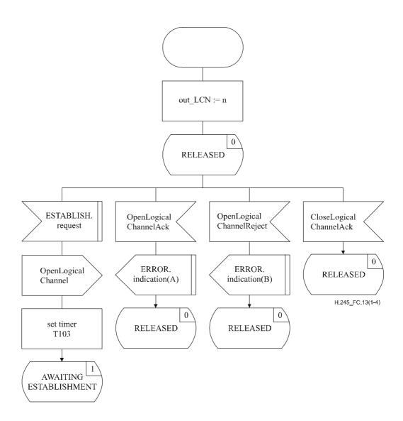
Figure C.13/H.245 – Outgoing LCSE SDL (sheet 1 of 4)
