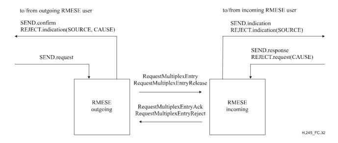
Figure C.32/H.245 – Primitives and messages in the Request Multiplex Entry Signalling Entity
