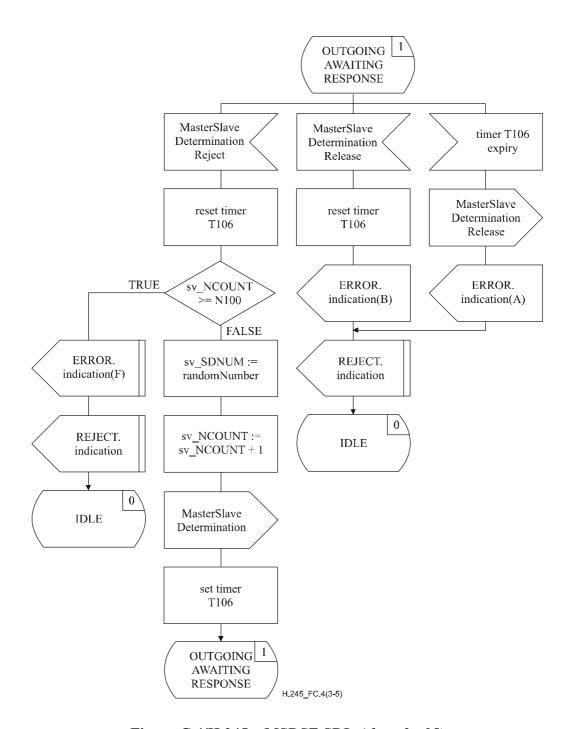
Figure C.4/H.245 – MSDSE SDL (sheet 3 of 5)
