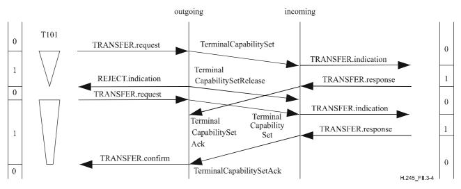
NOTE – The TerminalCapabilitySetRelease message arrives at the incoming CESE after response from the incoming CESE user. At the outgoing CESE the TerminalCapabilitySetAck message in response to the first TerminalCapabilitySet message is ignored. Only the second capability exchange is successful.
