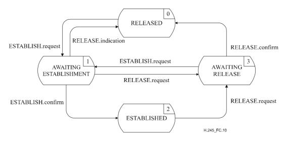
Figure C.10/H.245 – State transition diagram for sequence of primitives at outgoing LCSE
