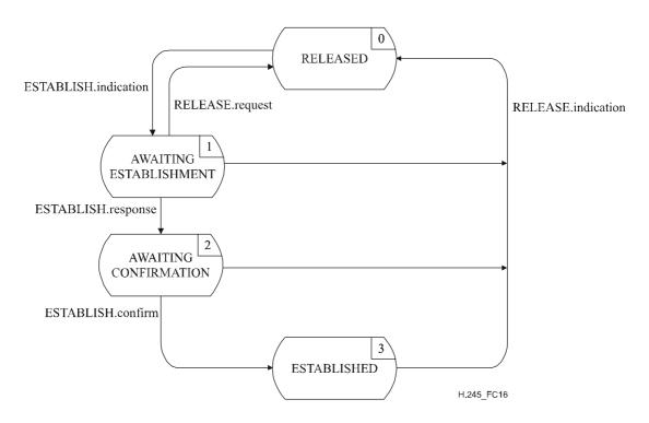
Figure C.16/H.245 – State transition diagram for sequence of primitives at incoming B-LCSE
