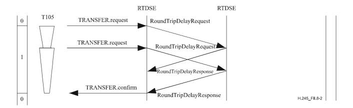
Figure II.8-2/H.245 – Round-trip delay determination procedure with an earlier unacknowledged round-trip delay procedure outstanding
