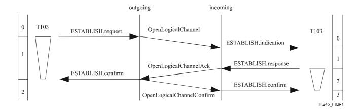
Figure II.9-1/H.245 – Bidirectional logical channel establishment
