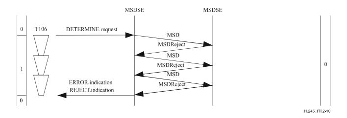
Figure II.2-10/H.245 – Master-slave determination – Indeterminate result with N100 = 3
