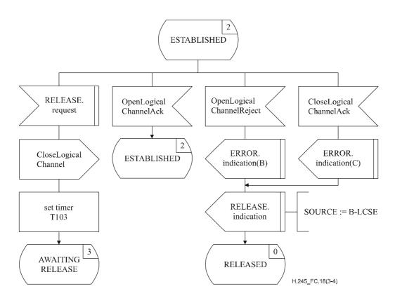
Figure C.18/H.245 - Outgoing B-LCSE SDL (sheet 3 of 4)
