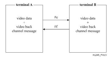
Figure VI.3/H.245 – Logical Channels for VideoMux Mode
