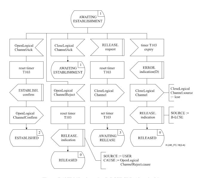
Figure C.18/H.245 - Outgoing B-LCSE SDL (sheet 2 of 4)
