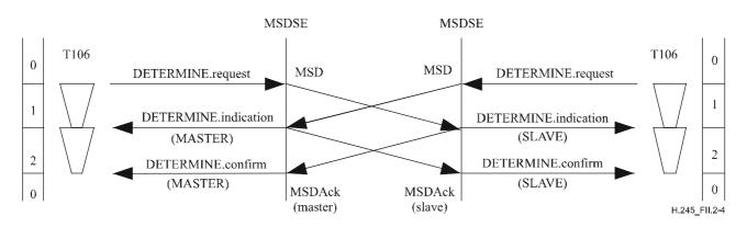
Figure II.2-4/H.245 – Master-slave determination – Simultaneous determination
