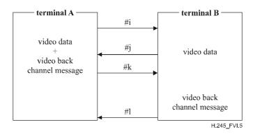
Figure VI.5/H.245 – Coexistence of Separate Logical Channel mode with VideoMux mode
