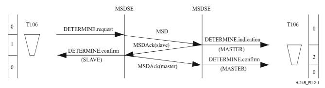
Figure II.2-1/H.245 – Master-slave determination – Master at remote MSDSE
