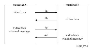
Figure VI.2/H.245 – Logical Channels for Separate Logical Channel Mode
