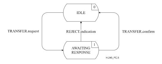
Figure C.5/H.245 – State transition diagram for sequence of primitives at outgoing CESE
