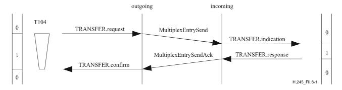
Figure II.6-1/H.245 – Successful multiplex table send request
