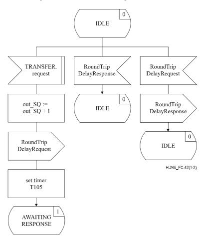
**Figure C.42/H.245 – RTDSE SDL** (*sheet 1 of 2*)
