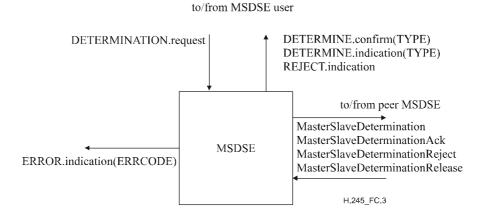
Figure C.3/H.245 – Primitives and messages in the MSDSE
