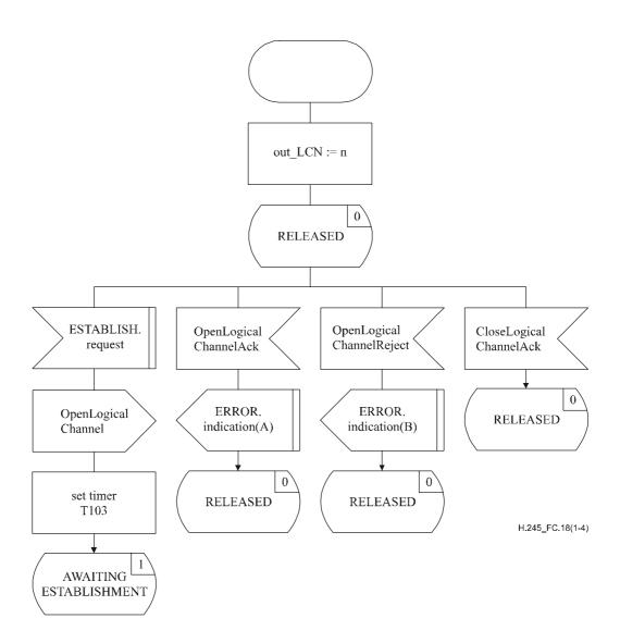
Figure C.18/H.245 – Outgoing B-LCSE SDL (sheet 1 of 4)
