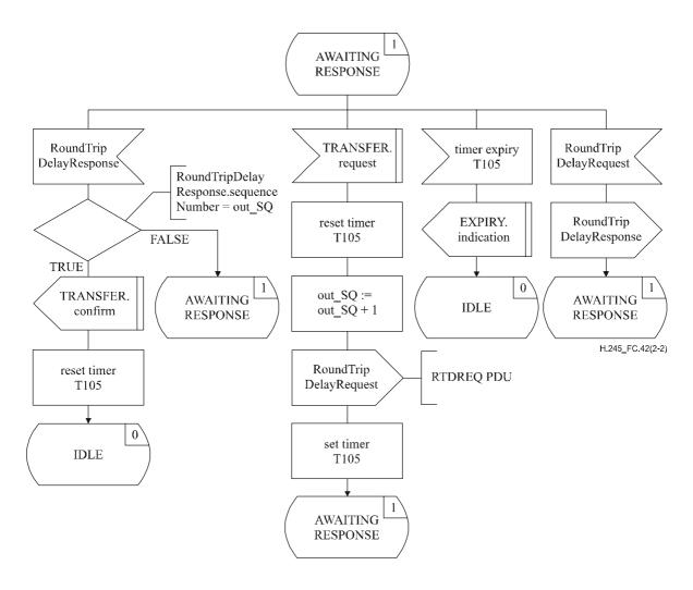
Figure C.42/H.245 – RTDSE SDL (sheet 2 of 2)
