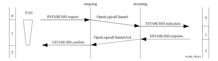
Figure II.4-1/H.245 – Logical channel establishment
