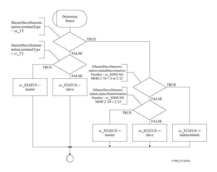
Figure C.4/H.245 – MSDSE SDL (sheet 5 of 5)
