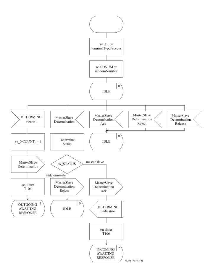
Figure C.4/H.245 – MSDSE SDL (sheet 1 of 5)
