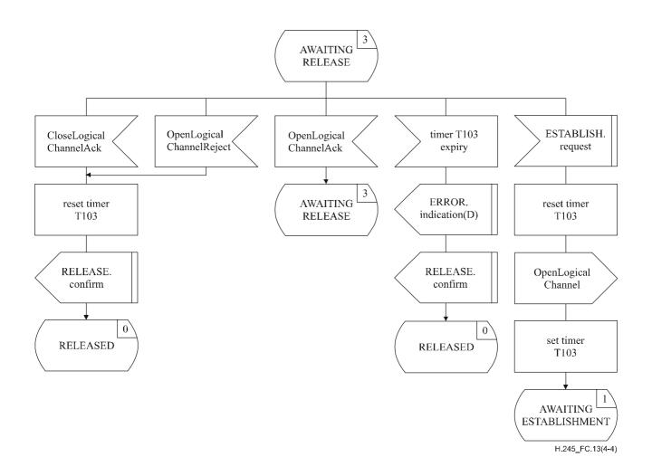
Figure C.13/H.245 – Outgoing LCSE SDL (sheet 4 of 4)
