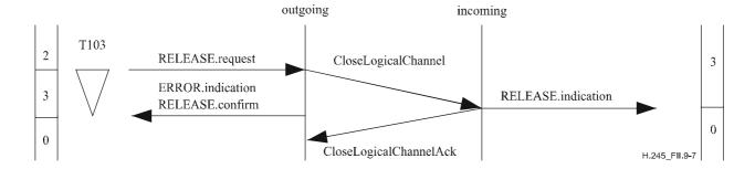
Figure II.9-7/H.245 – Bidirectional logical channel release request with expiry of timer T103 at the outgoing side
