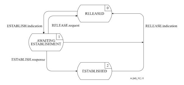
Figure C.11/H.245 – State transition diagram for sequence of primitives at incoming LCSE
