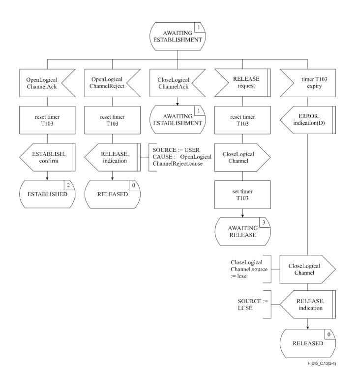
Figure C.13/H.245 – Outgoing LCSE SDL (sheet 2 of 4)
