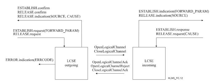
Figure C.12/H.245 – Primitives and messages in the Logical Channel Signalling Entity
