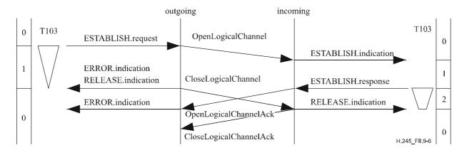
NOTE – Timer T103 at the outgoing side has expired after transmission of the OpenLogicalChannelAck message at the incoming B-LCSE, but before reception of the OpenLogicalChannelAck message at the outgoing B-LCSE.
