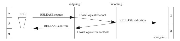
Figure II.4-2/H.245 – Logical channel release
