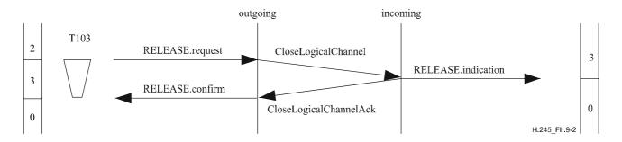
Figure II.9-2/H.245 – Bidirectional logical channel release
