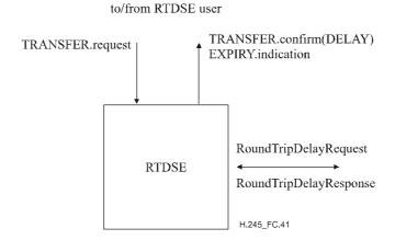
Figure C.41/H.245 – Primitives and messages in the RTDSE
