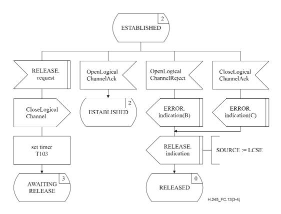
Figure C.13/H.245 – Outgoing LCSE SDL (sheet 3 of 4)
