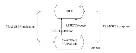
Figure C.6/H.245 – State transition diagram for sequence of primitives at incoming CESE
