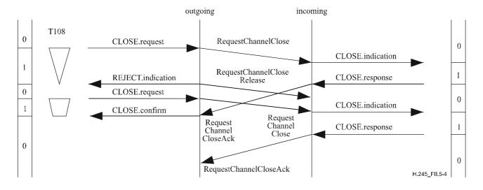
NOTE – The close channel request is confirmed on reception of the first RequestChannelClose message.
