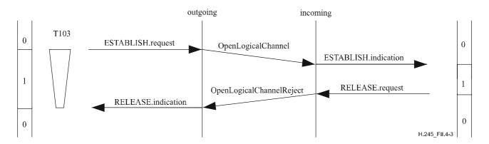
Figure II.4-3/H.245 – Logical channel establishment rejection by peer LCSE user
