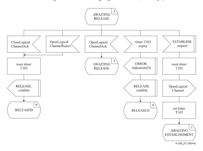
Figure C.18/H.245 – Outgoing B-LCSE SDL (sheet 4 of 4)
