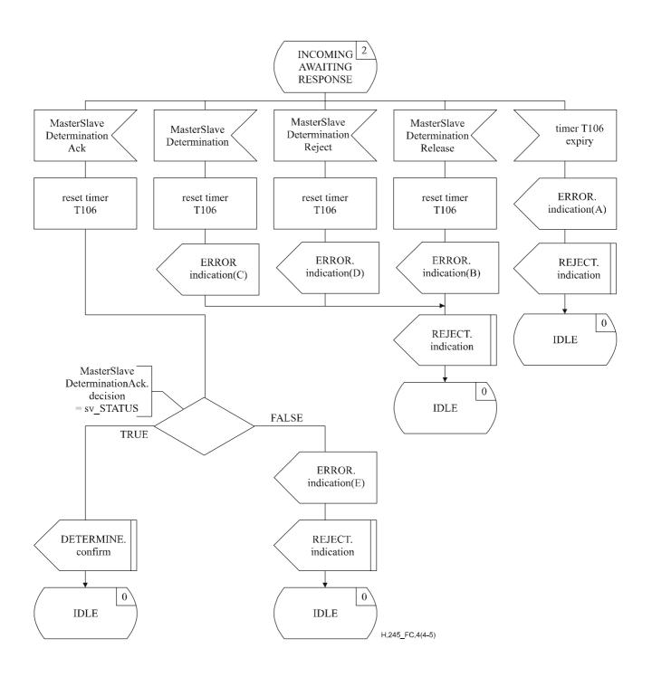
Figure C.4/H.245 – MSDSE SDL (sheet 4 of 5)
