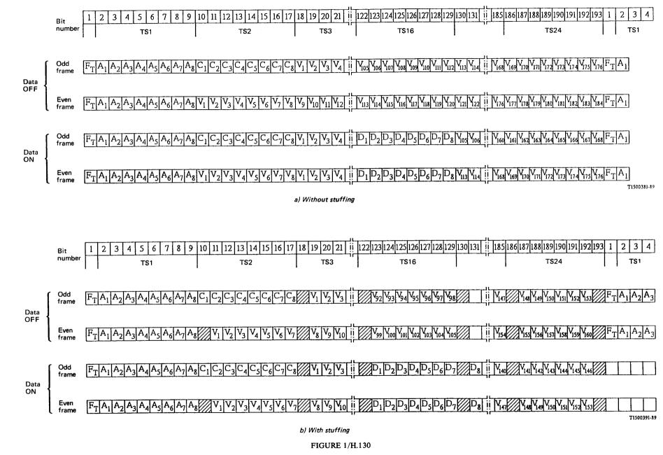
Frame structure and bit allocation
