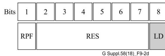
Figure 9-2d – Optional Rx line pre-FEC local degrade status bit location in the first instance of FlexO OH STAT field (Rx ODSP to framer direction)
