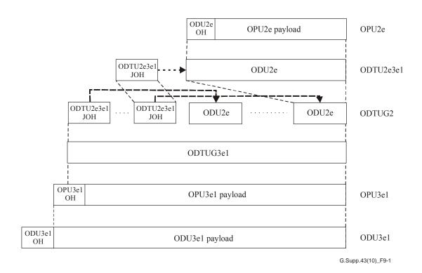
Figure 9-1 – ODU2e into ODU3e1 multiplexing method
