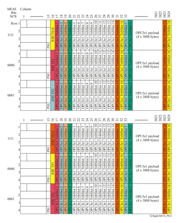
Figure 9-2 – OPU3e1 tributary slot allocation
