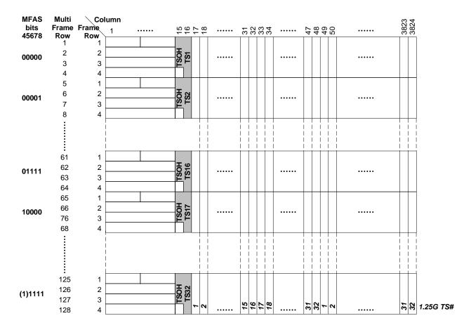
Figure 9-8 – OPU3e2 tributary slot allocation
