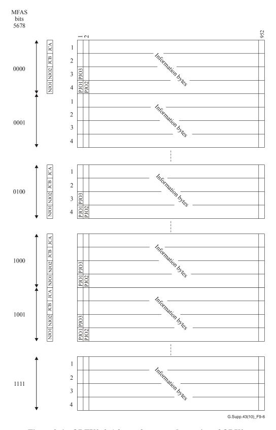
Figure 9-6 – ODTU2e3e1 frame format and mapping of ODU2e
