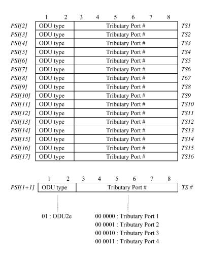
Figure 9-5 – MSI coding for ODU3e1
