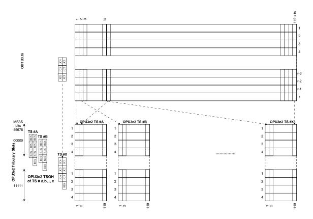
Figure 9-9 - Mapping of ODTU3e2.ts into 'ts' OPU3e2 1.25G tributary slots
