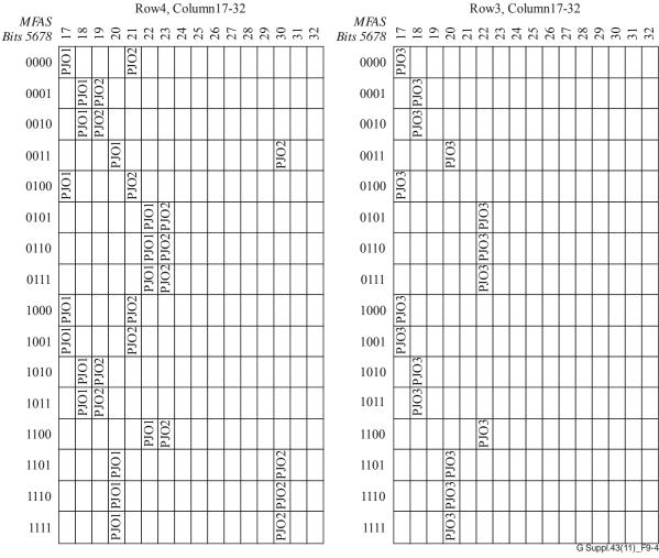
Figure 9-4 - OPU3e1 multiplex overhead
