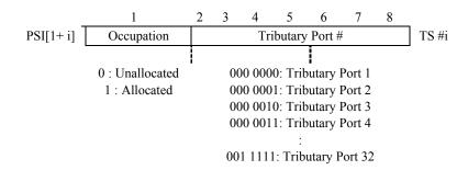
Figure 9-11B - OPU3e2 MSI coding - Payload type 21
