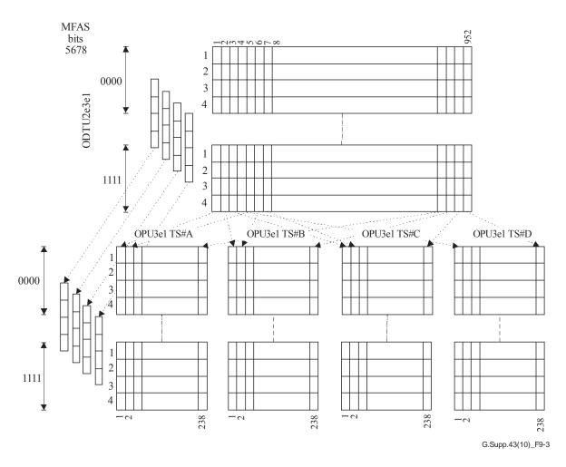
Figure 9-3 – Mapping of ODTU2e3e1 (excluding JOH) into four OPU3e1 TribSlots (#A, #B, #C, #D with A<B<C<D)
