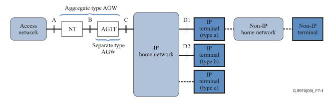
Figure 7-1 – Possible demarcation points for IP terminals
