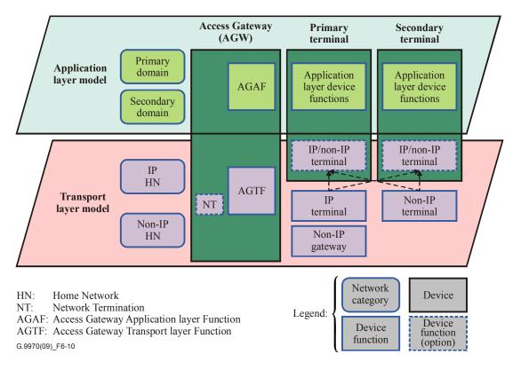
Figure 6-10 – The conceptual diagram of two layered generic home network models
