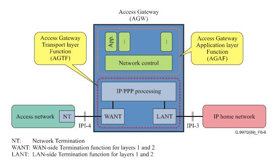
**Figure 6-6 – Decomposition of access gateway**
