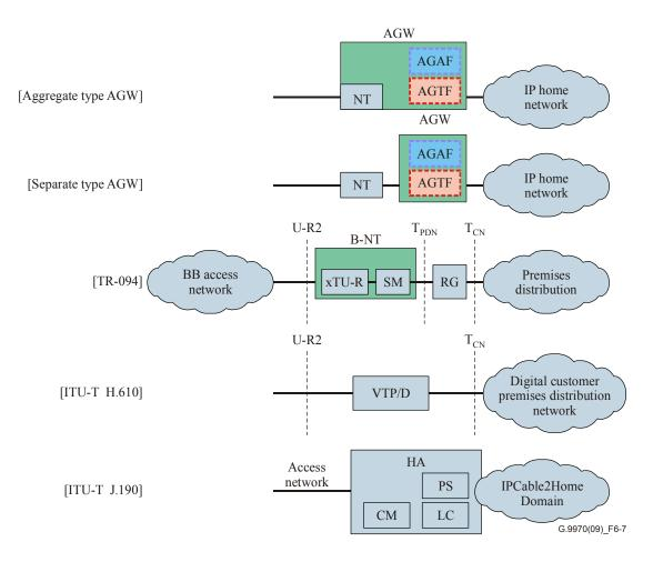
Figure 6-7 – The configuration of AGW in comparison with some documents
