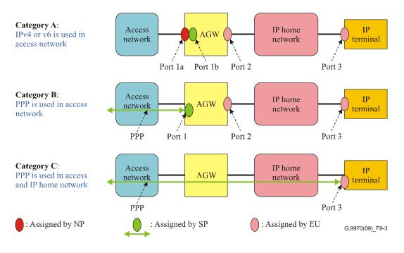
Figure 8-3 – Examples of IP addressing schemes
