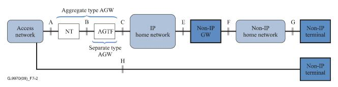
Figure 7-2 – Possible demarcation points for non-IP terminals
