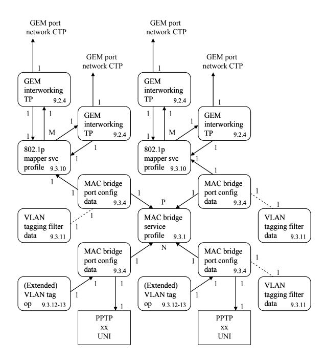
Figure 8.2.2-9 – Illustration of N:MP bridge-map-filtering
