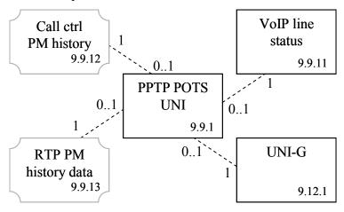
Figure 8.2.8-2 – IP path managed ITU-T H.248 VoIP
