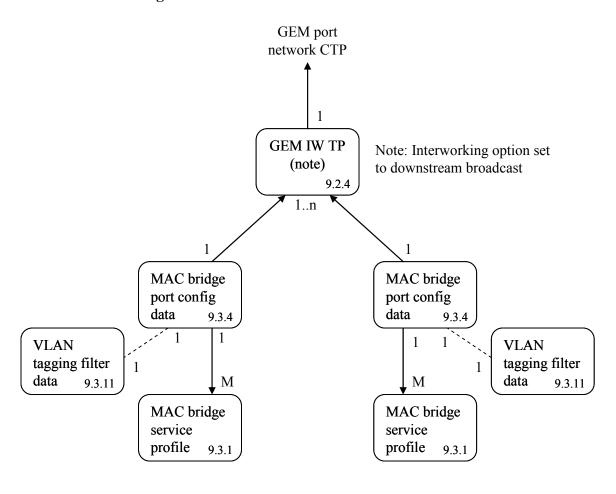
Figure 8.2.2-11 – Illustration of downstream broadcast configuration
