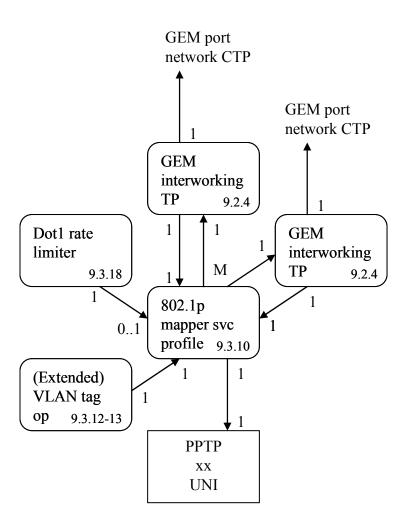
Figure 8.2.2-4 – Illustration of 1:M mapping
