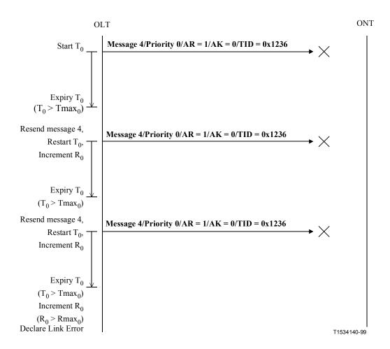
Figure 11.3-2 – OMCC link error detection
