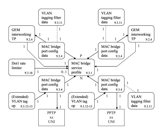
Figure 8.2.2-8 – Illustration of N:P bridge-filtering
