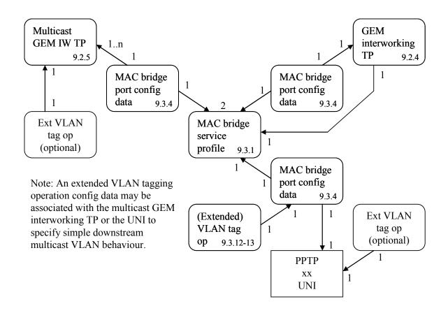
Figure 8.2.2-10 – Illustration of multicast service
