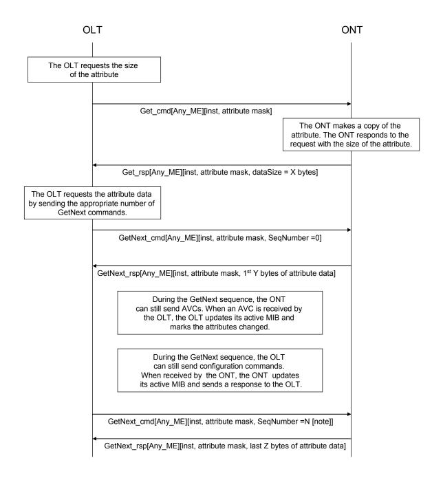
NOTE – N+1 is the number of get next commands as derived by the OLT to retrieve the complete table. For baseline OMCI messages, Y is 29 bytes; for extended OMCI messages, Y = 1966 Bytes (1980 PDU size – 14 Bytes of OMCI header).
