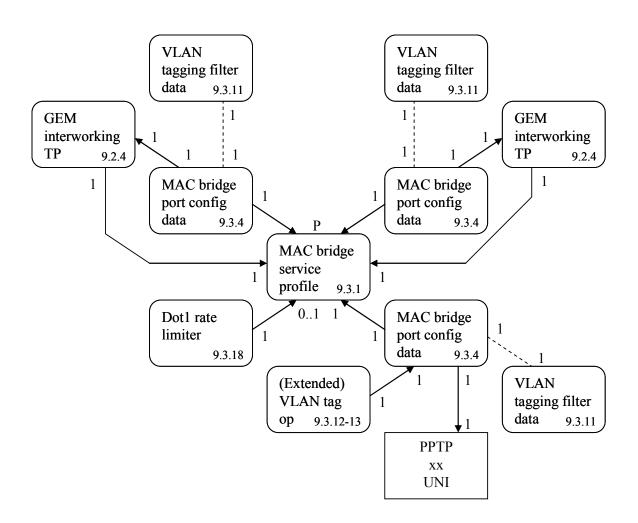
Figure 8.2.2-5 – Illustration of 1:P filtering
