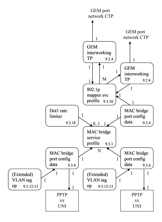
Figure 8.2.2-6 – Illustration of N:M bridge-mapping
