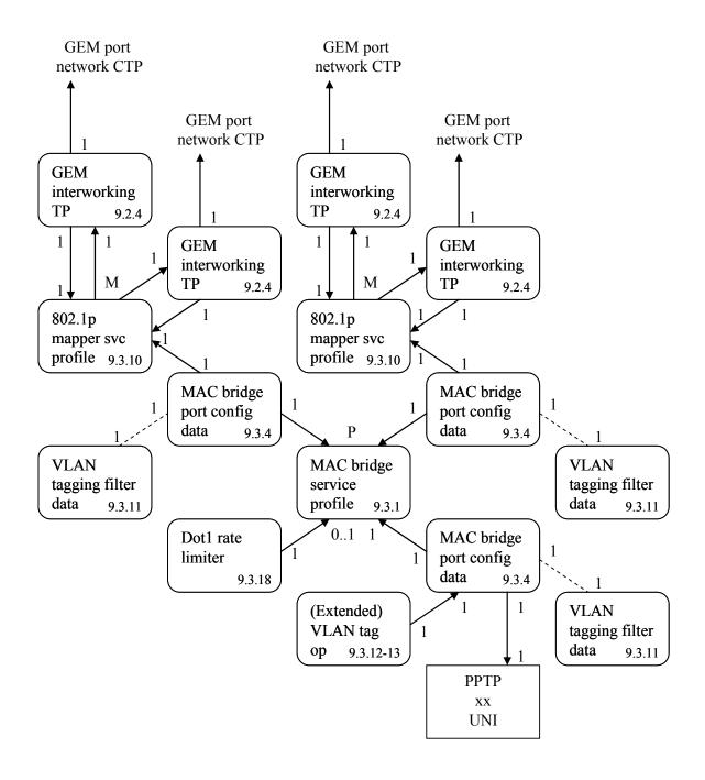
Figure 8.2.2-7 – Illustration of 1:MP map-filtering
