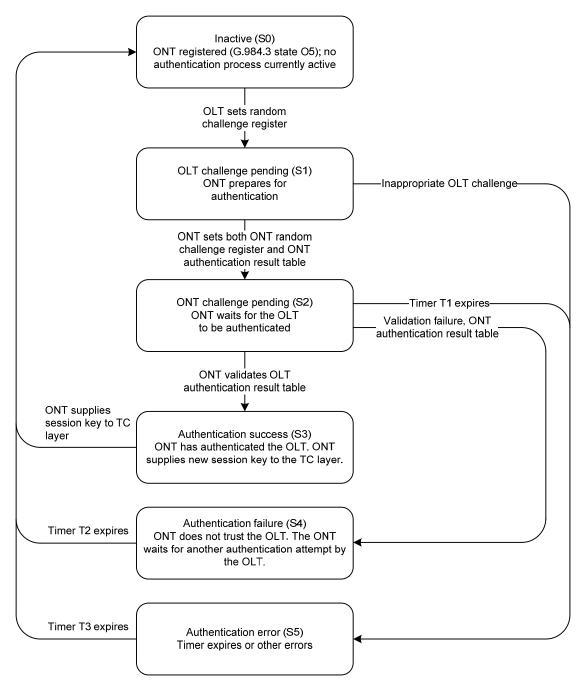
NOTE 1 – Timer T1 – ONT challenge pending timer. Timer T1 is used to abort an unsuccessful OLT authentication attempt by limiting the overall time an ONT can remain in state S2. The recommended value of T1 is 3 seconds.
