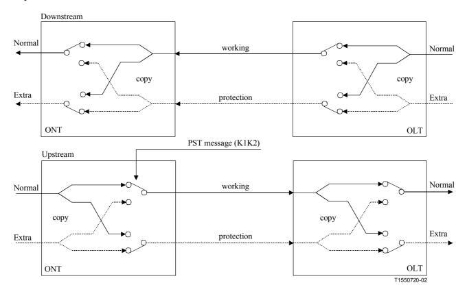
Figure 9/G.983.5 – 1:1 switching architecture
