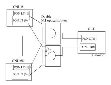
Figure 2/G.983.5 - Type C: Fully protected system, 1:1 and 1+1
