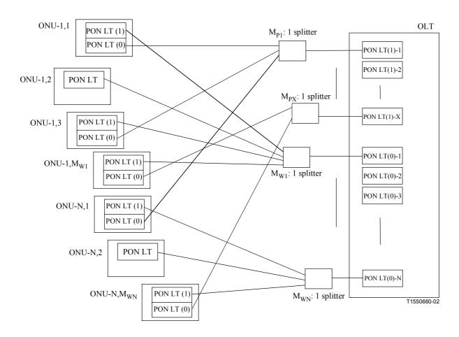
Figure 3/G.983.5 – Type C: X:N protection system
