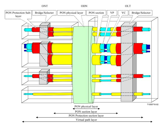
Figure 8/G.983.5 – The layer image in B-PON
