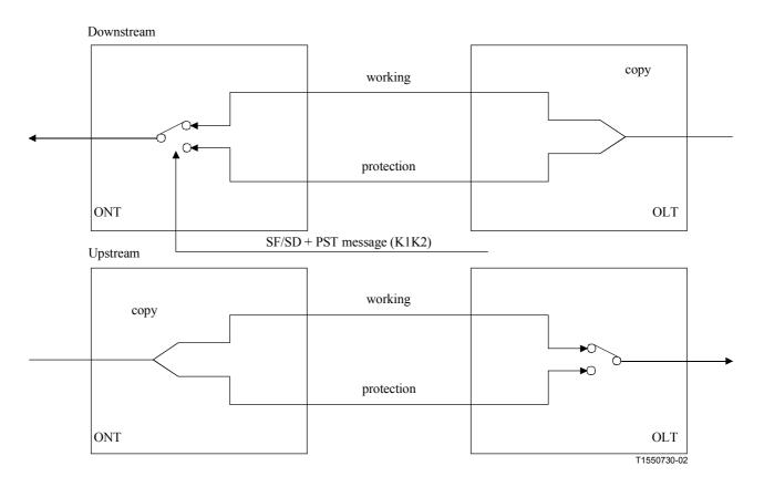
Figure 10/G.983.5 – 1+1 switching architecture
