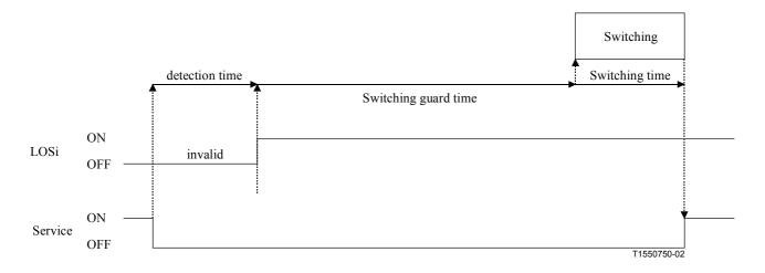
Figure 12/G.983.5 – Protection switching typical model (Without POPUP procedure)
