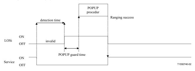
Figure 11/G.983.5 – Protection switching typical model (With POPUP procedure)
