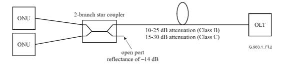
Figure I.2/G.983.1 – Effect of open connectors located at OLT side of star coupler
