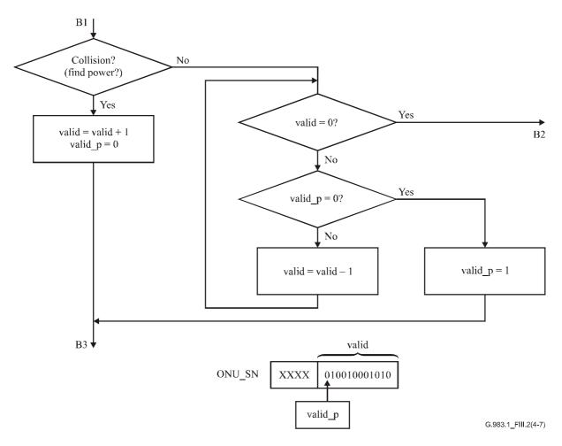
NOTE – The points of B1, B2 and B3 correspond to the points of B1, B2 and B3 in Figure III.2 respectively. "valid" means the number of valid bits of ONU serial number. "valid p indicates the bit of the most significant bit of valid bits.
