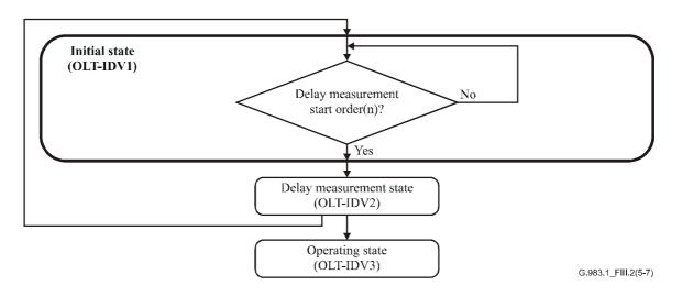
Figure III.2/G.983.1 – Ranging flow [OLT] (example) (sheet 5 of 7)
