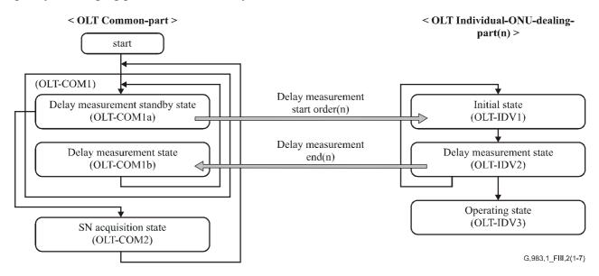
Figure III.2/G.983.1 – Ranging flow [OLT] (example) (sheet 1 of 7)
