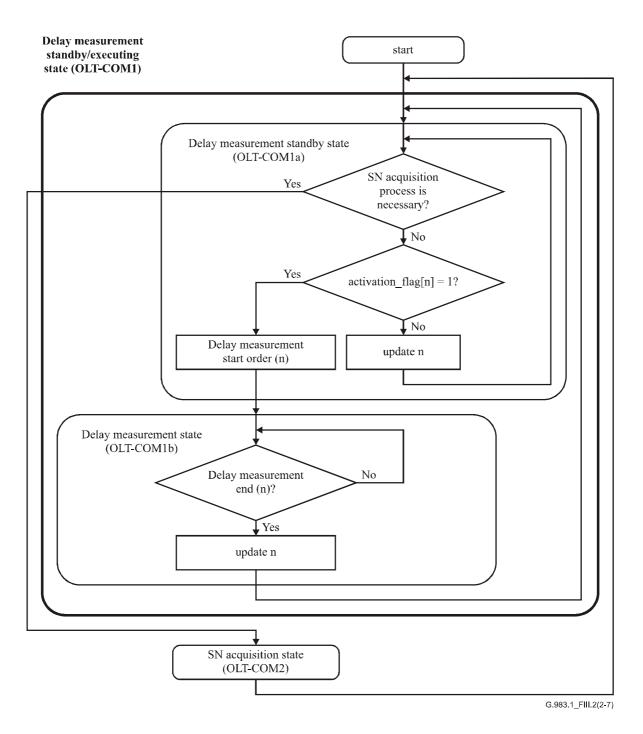
Figure III.2/G.983.1 – Ranging flow [OLT] (example) (sheet 2 of 7)
