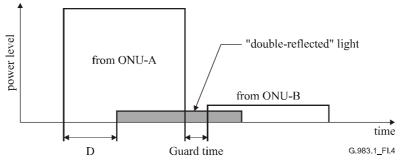
D Round-trip time between ONU-A and connector-C.
