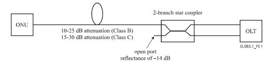
Figure I.1/G.983.1 – Effect of open connectors located at ONU side of star coupler
