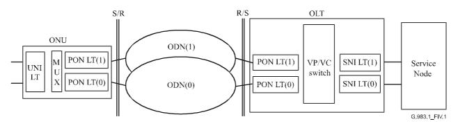
Figure IV.1/G.983.1 – Duplex system model
