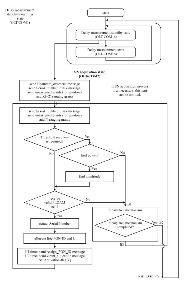
Figure III.2/G.983.1 - Ranging flow [OLT] (example) (sheet 3 of 7)
