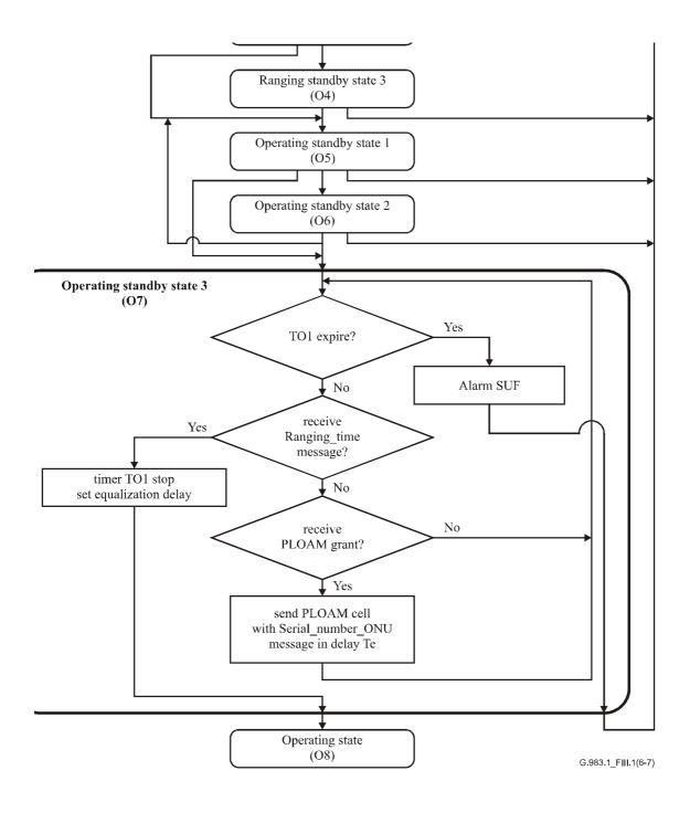
Figure III.1/G.983.1 – Ranging flow [ONU] (example) (sheet 6 of 7)
