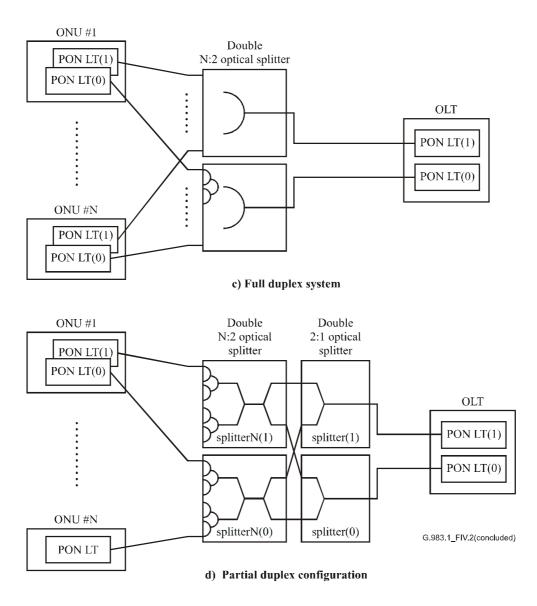
Figure IV.2/G.983.1 – Duplex ATM-PON system (concluded)
