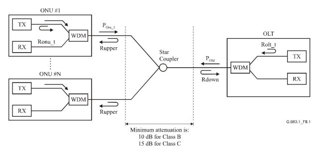
Figure II.1/G.983.1 – Reflectance model to be considered
