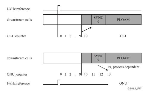
Figure 17/G.983.1 – 1-kHz reference extraction in ONU
