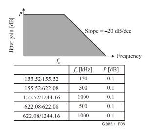
Figure 8/G.983.1 – Jitter transfer for ONU
