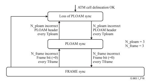
Figure 16/G.983.1 – Frame synchronization flow
