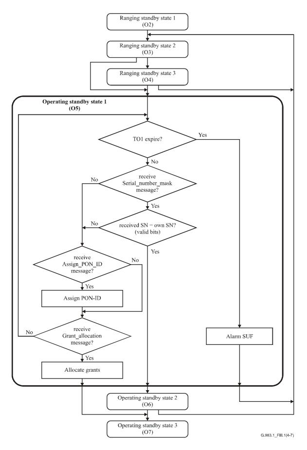
Figure III.1/G.983.1 – Ranging flow [ONU] (example) (sheet 4 of 7)
