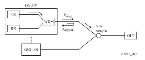
Figure II.2/G.983.1 – Model for incidence into ONU receiver
