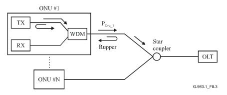
Figure II.3/G.983.1 – Model 1 for incidence into OLT receiver
