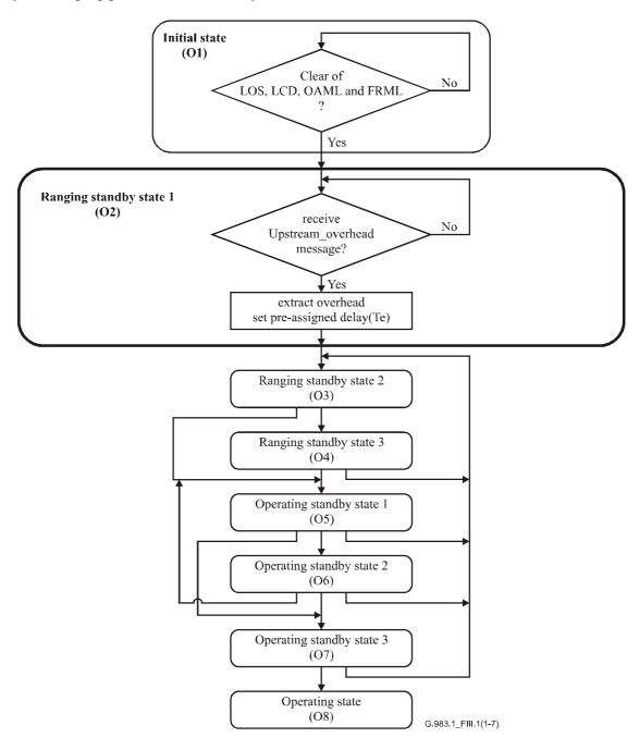
Figure III.1/G.983.1 – Ranging flow [ONU] (example) (sheet 1 of 7)
