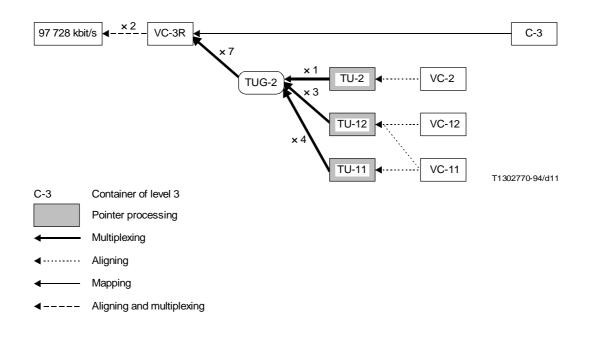
NOTE - The VC-3R is a VC-3 SDH element with reduced functionality as shown in Figure 2-4.
