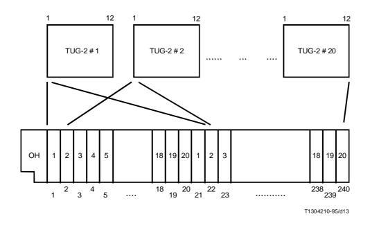
FIGURE 3-7/G.832 Multiplexing of 20 × TUG-2 info the 139 264 kbit/s payload capacity
