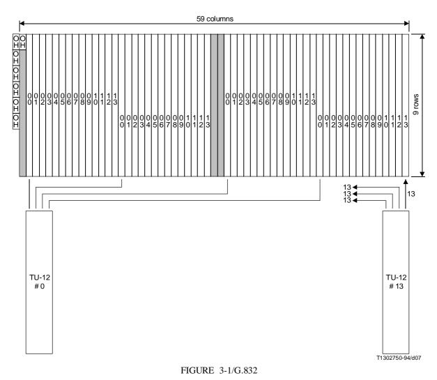
Support of 14 TU-12 s in the 34 368 kbit/s frame structure
