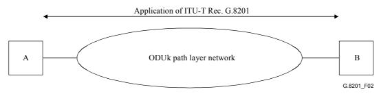
NOTE - A and B are path end points located at the path terminations as defined in ITU-T Rec. G.798 [2].
