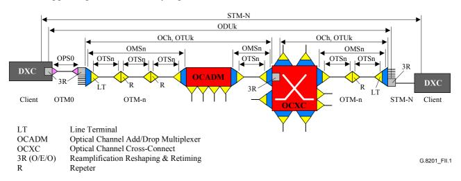
Figure II.1/G.8201 – Example of the transport of an STM-N signal in OTN
