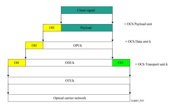
Figure 1/G.8201 – OTN signal structure
