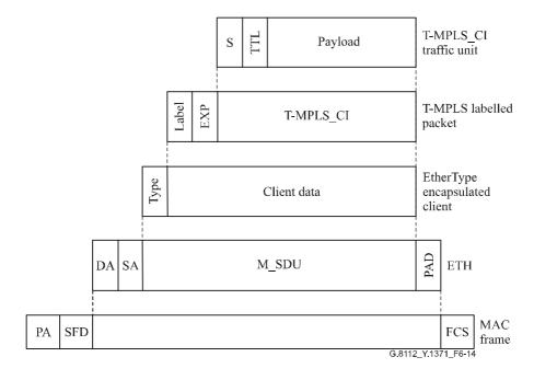
Figure 6-14 – Type encapsulation ETH link frame
