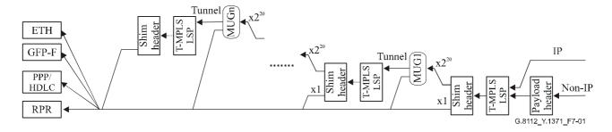
Figure 7-1 – T-MPLS mapping, multiplexing and segment monitoring
