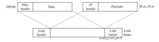
Figure 6-17 – T-MPLS control frame over shared trail SCN links
