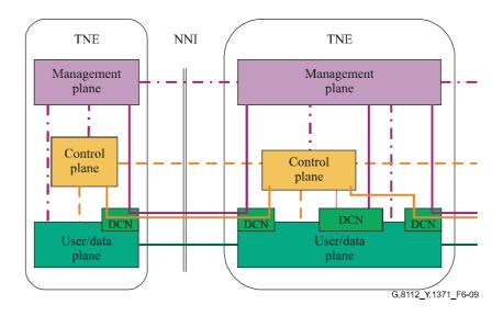
Figure 6-9 – Three planes of T-MPLS NNI
