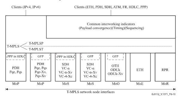
Figure 6-10 – Structure of the T-MPLS network node interfaces
