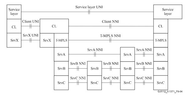
Figure 6-4 – Example of layer networks in client UNI and T-MPLS NNI in case of access link to a client's layer service node
