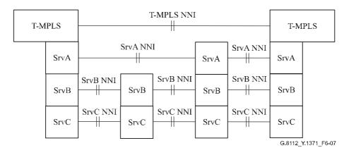
Figure 6-7 – Example of layer networks in T-MPLS NNI in case of interconnecting two T-MPLS layer service nodes
