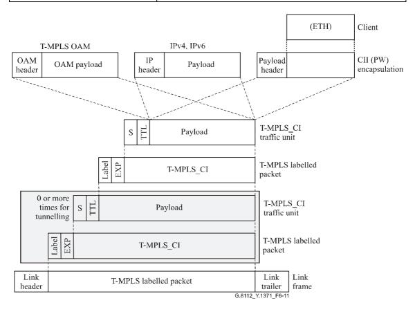
Figure 6-11 – T-MPLS principle information containment
