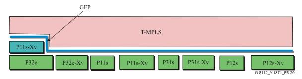
Figure 6-20 – Components of the T-MPLS over PDH NNI using GFP-F
