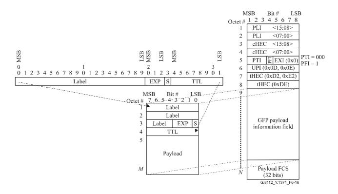
Figure 6-16 – Mapping T-MPLS labelled packet into GFP-F link frame
