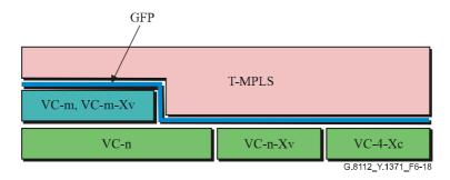
Figure 6-18 – Components of the T-MPLS over SDH NNI using GFP-F encapsulation
