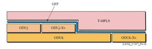
Figure 6-19 – Components of the T-MPLS over OTH NNI
