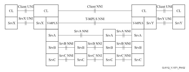
Figure 6-2 – Example of layer networks in client UNI and T-MPLS NNI in case of pt-pt T-MPLS layer connection
