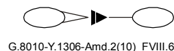
Figure VIII.6 – Layer transitional link with two client link points and one server link point
