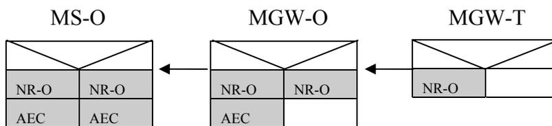
**Figure I.8 – Reverse capability list exchange and update, from MGW-T to MS-O**
