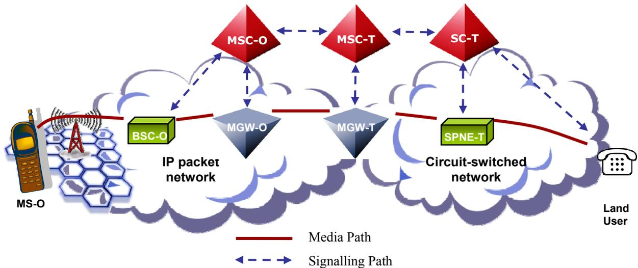
**Figure I.6 – Mobile-to-land call through an IP packet network and a circuit-switched network**
