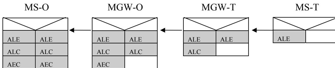
**Figure I.3 – Reverse capability list exchange and update, from MS-T to MS-O**
