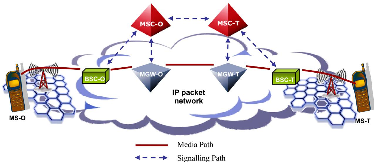
Figure I.1 – Mobile-mobile non-transcoder free operation VoIP call
