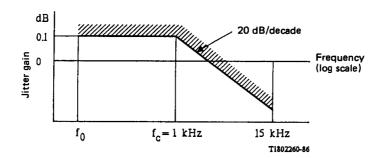
$\it Note$  - The frequency  $f_0$  should be as low as possible, taking into account the limitations of measuring equipment In any case  $f_0$  should be no greater than 10 Hz. The selective measurement method should be used.
