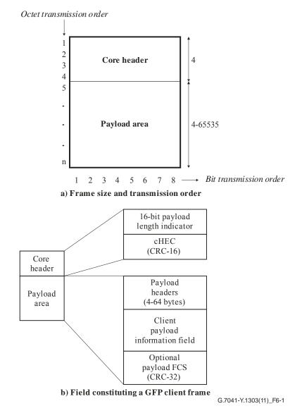
Figure 6-1 – Frame format for GFP client frames
