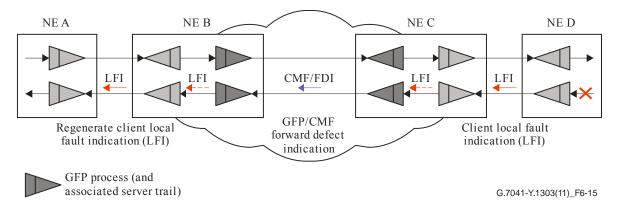
Figure 6-15 – Examples a forward defect indication of a client link fault status indication
