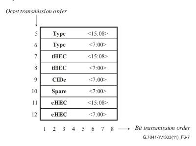
Figure 6-7 – Payload header for a linear (point-to-point) frame including the extension header
