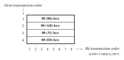
Figure 6-11 – GFP idle frame (Barker-like scrambled frame)
