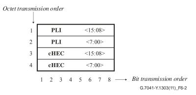
Figure 6-2 – GFP core header format
