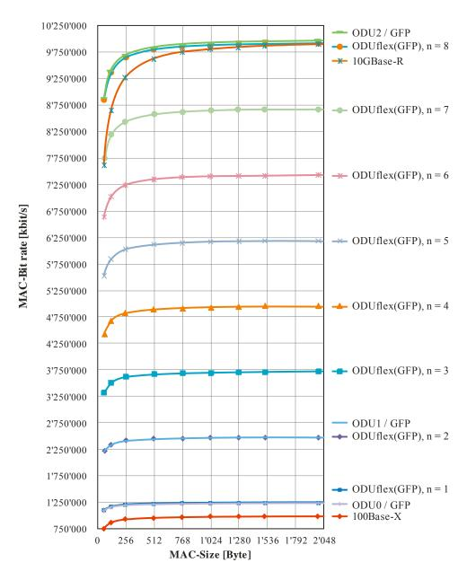
Figure VII.1 – Packet data throughput for ODUflex(GFP), n=1,...,8, ODUk (k=0,1,2), 1000Base-X, 10GBase-R
