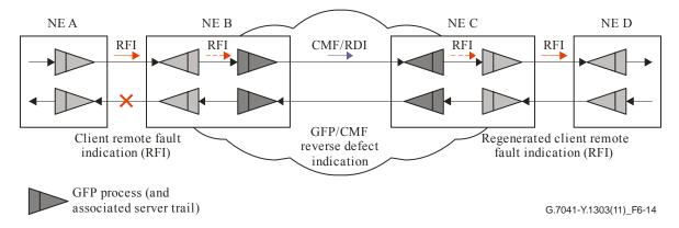
Figure 6-14 – Examples of a reverse defect indication of a client link fault status indication
