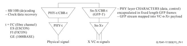
Figure I.1 – FC/ES/FI/GE tributary interface port using full-rate GFP-T mapping in SDH network element
