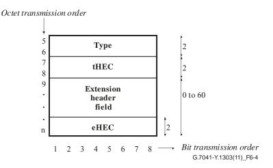
Figure 6-4 – GFP payload header format
