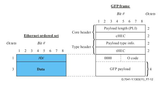
Figure 7-12 – Ethernet ordered set mapping into GFP-F
