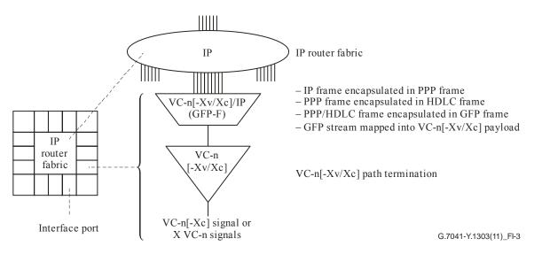
Figure I.3 – VC-n/VC-n-Xv/VC-n-Xc port on IP router or IP router function embedded in hybrid SDH/IP equipment
