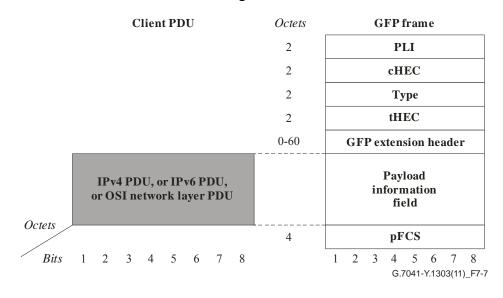
Figure 7-7 – IPv4/IPv6/OSI network layer PDUs and GFP frame relationships
