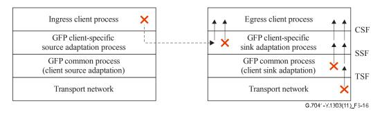
Figure 6-16 – Defect signal propagation in GFP
