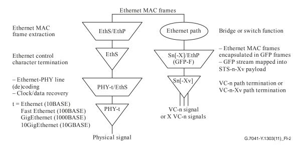
Figure I.2 – Ethernet tributary interface port using GFP-F mapping in SDH network element
