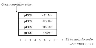
Figure 6-8 – GFP payload frame check sequence format
