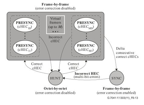
Figure 6-13 – GFP frame delineation state diagram
