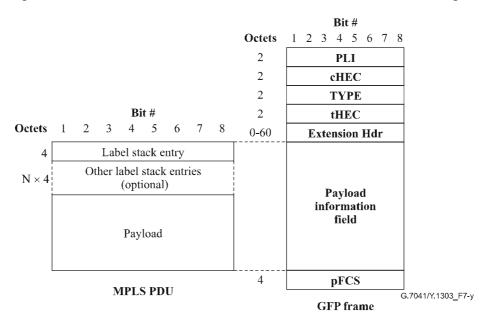
Figure 7-y/G.7041/Y.1303 – Unicast MPLS and GFP frame relationships
