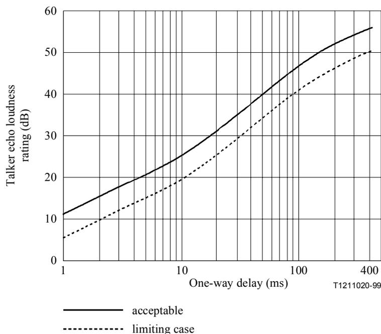
Acceptable: Equivalent to the curve with "1%" probability of encountering objectionable echo in Recommendation G.131.
