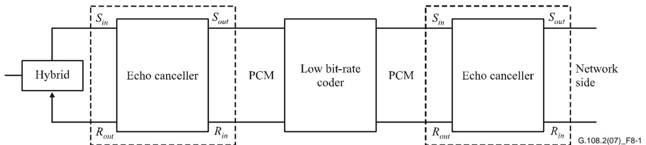
**Figure 8-1 – Low bit-rate coder between tandem cancellers**
