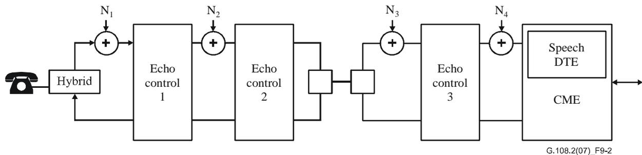
**Figure 9-2 – Multiple echo control devices in a CME network configuration**
