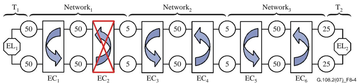
**Figure 8-4 – Example of connection via three concatenated networks including a private network**
