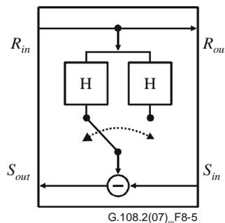
**Figure 8-5 – Possible implementation of echo canceller with two independent H echo-path estimators**
