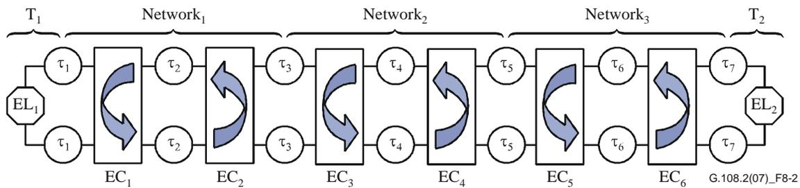
**Figure 8-2 – Reference connection for tandem ECs**
