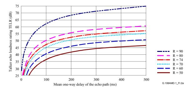
Figure I.2a/G.108 – Effects of talker echo based on E-model
