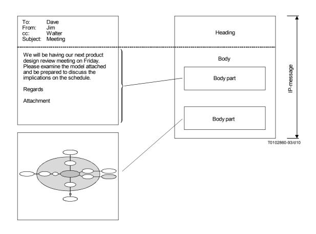
FIGURE 10/F.400 **IP-message structure for a typical memo**
