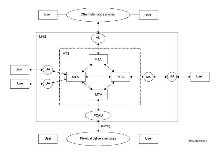
NOTE - Message input from PDS to MHS is for further study. Flow from PD services to the PDAU shown is for the purpose of notifications
