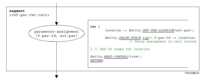
Figure B.71/Z.140 – Flow graph segment <ref-par-var-calc>
