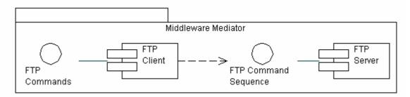
Figure D.2 - FTP Client-Server-Architecture
