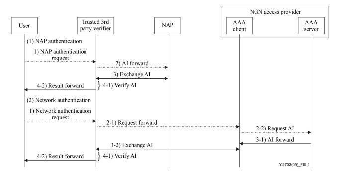
Figure III.4 – Procedure of user authentication and authorization of NGN providers
