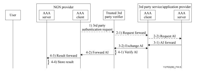
Figure III.5 – Procedure of NGN provider authentication and authorization of 3rd party service/application provider
