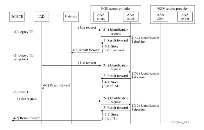
Figure III.1 – Procedure of identification for a device to access NGN network
