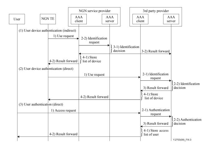
Figure III.3 – Procedure of NGN service provider authentication and authorization of user
