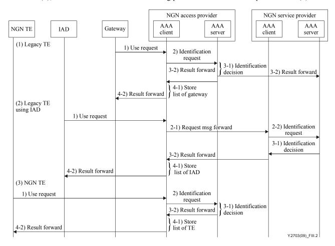
Figure III.2 – Procedure of identification for a device to use service/application provider
