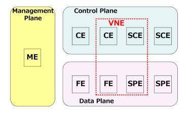
Figure 6-1 – Three planes and reconstructible components
