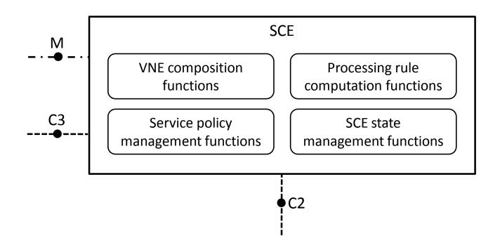
**Figure 6-4 – Service control element**
