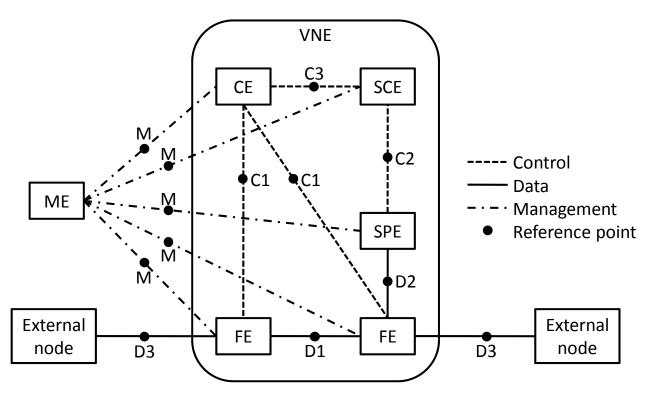
Figure 6-2 – iSCP functional architecture
