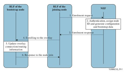
Figure I.1 – Control node enrolment to DHT-based overlay in the DSN network
