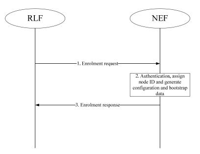
Figure 7-2 – DSN node (with the RLF) enrolling to the DHT-based overlay
