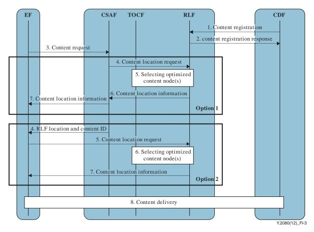
Figure I.3 – Providing content delivery services
