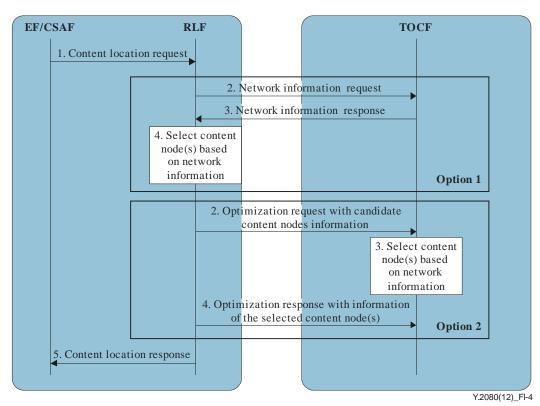
**Figure I.4 – Selecting optimized content node(s)**
