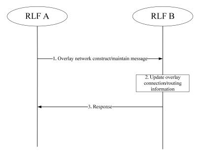
Figure 7-3 – Exchanging information to construct and maintain the overlay
