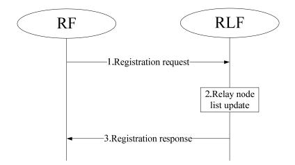
Figure 7-11 – Relay node registration
