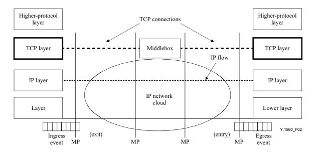
Figure 2/Y.1560 – Relationship between reference events and measurement points
