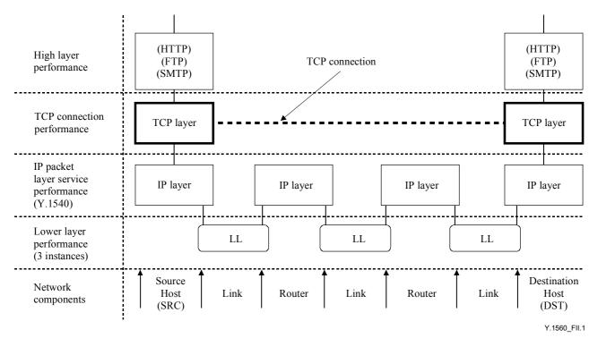
Figure II.1/Y.1560 – Layered model of performance for TCP connection without a middlebox – example
