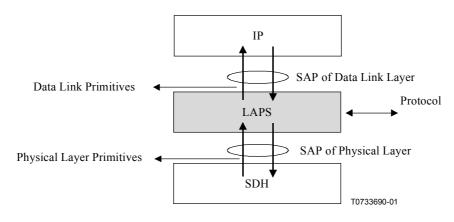
Figure 1/X.85/Y.1321 – The relationship between LAPS and IP, LAPS and SDH
