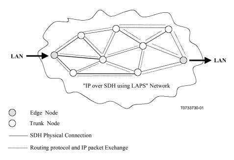
Figure 5/X.85/Y.1321 – "IP over SDH using LAPS" network example
