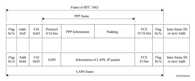
Figure I.1/X.85/Y.1321 – The frame format comparison of LAPS in ITU-T X.85/Y.1321 with PPP/HDLC in RFC 1662
