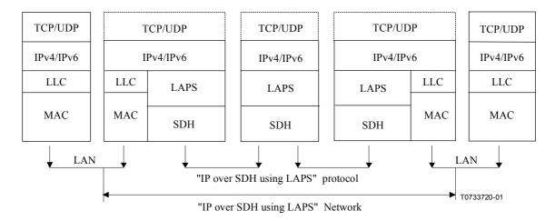
Figure 4/X.85/Y.1321 – The Protocol Configuration of IP over SDH using LAPS
