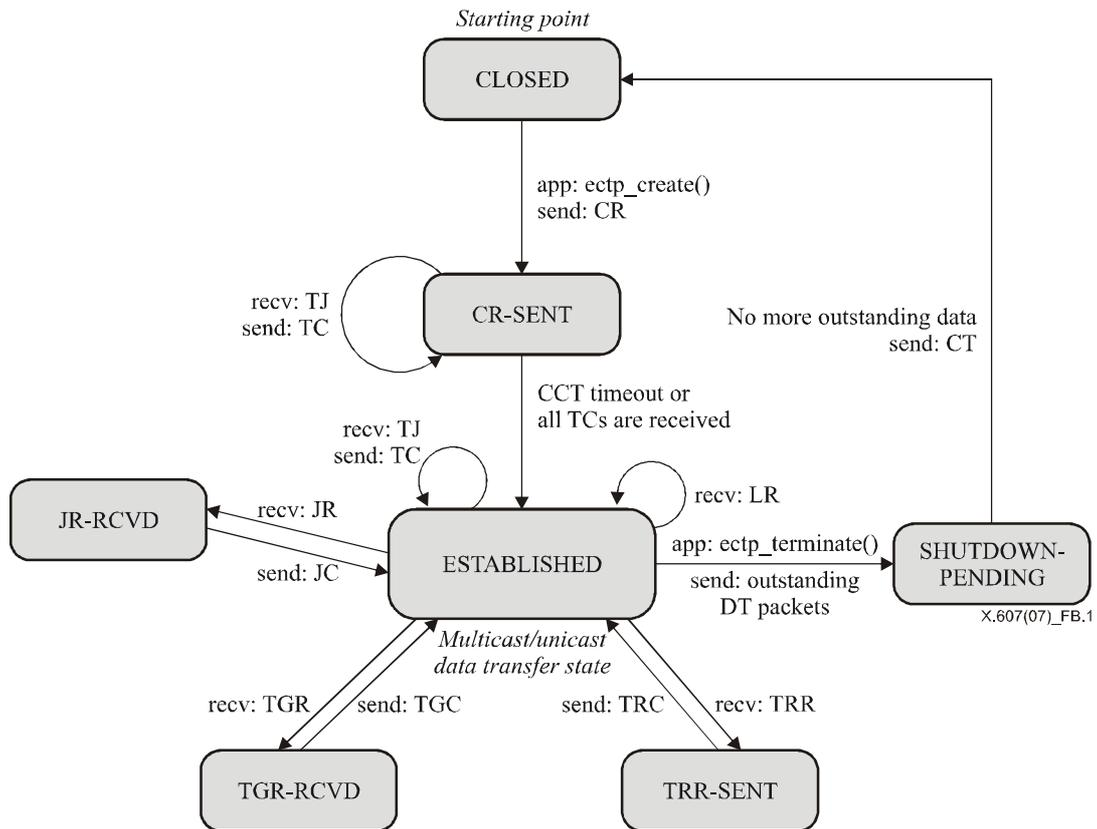
**Figure B.1 – State transition diagram for ECTP-3 TO**
