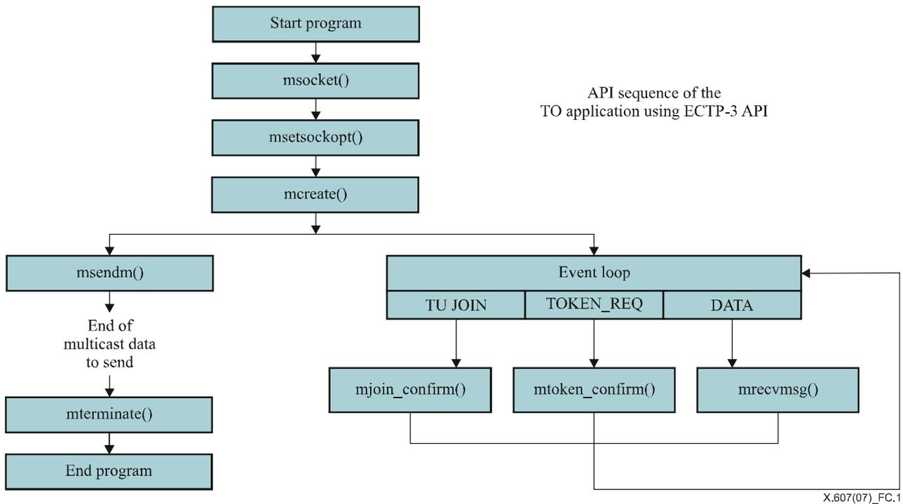
Figure C.1 – Example sequence of ECTP-3 APT functions called by TO
