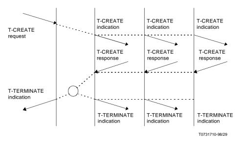
Figure 28 – Sequence of primitives in TS-provider rejection of a TC Creation attempt due to incomplete TC-characteristics
