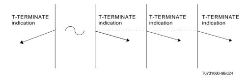
Figure 23 – Sequence of primitives in TS-provider invocation of a TC termination
