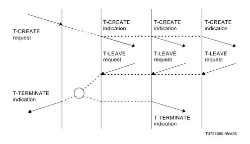
Figure 25 – Sequence of primitives in an unsuccessful TC Creation with multiple TS-user rejection(s)
