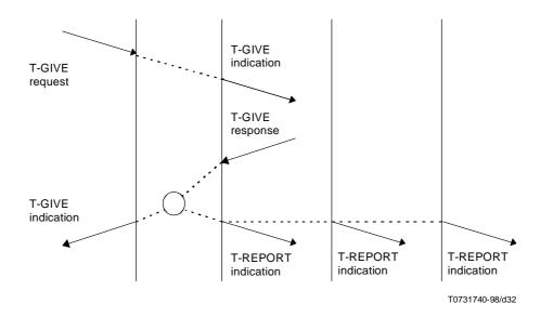
Figure 31 – Sequence of primitives in a token distribution to a specified TS-user by a TC-owner
