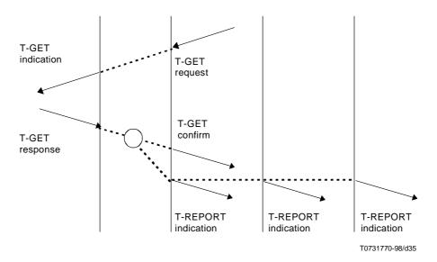
Figure 34 – Sequence of primitives in a token acquisition by a specified TS-user from the TC-owner
