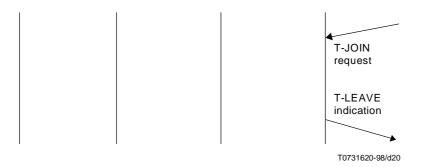
Figure 19 - Sequence of primitives in TS-provider rejection of a TC Join attempt
