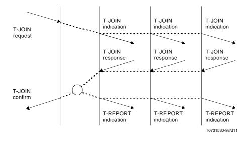
Figure 10 – Sequence of primitives in a successful TC Join by a focal TS-user
