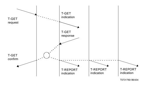
Figure 33 – Sequence of primitives in a forced token return from a specified TS-user by the TC-owner
