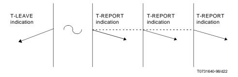
Figure 21 – Sequence of primitives in TS-provider expulsion of TS-user
