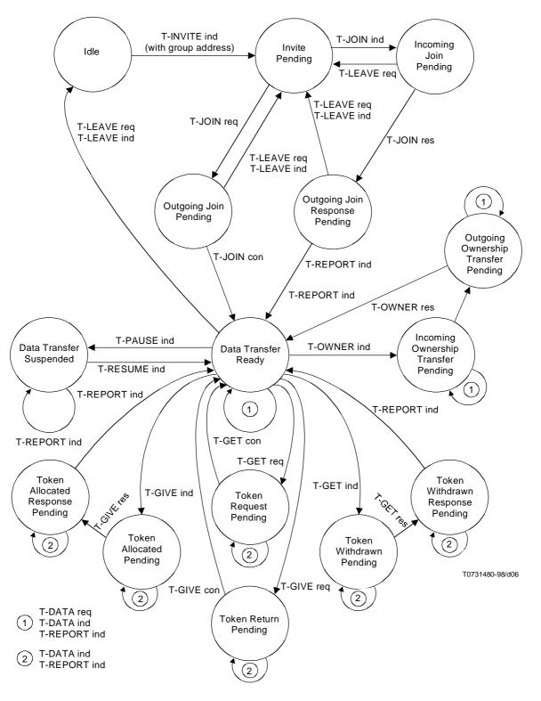
NOTE – T-TERMINATE request and/or indication may occur at any states, except the idle states, which then will lead to the Idle state. All states except the Data Transfer Suspended include a self-loop branch due to T-UNITDATA request and T-UNITDATA indication; these primitives may occur at such states without causing transition to other states.
