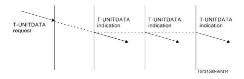
Figure 13 - Sequence of primitives in data transfer using T-UNITDATA primitives
