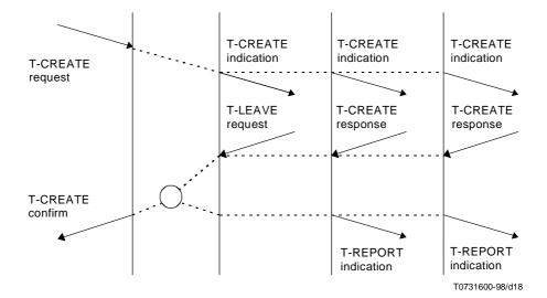
Figure 17 – Sequence of primitives in a successful TC Creation with some TS-user rejection(s)
