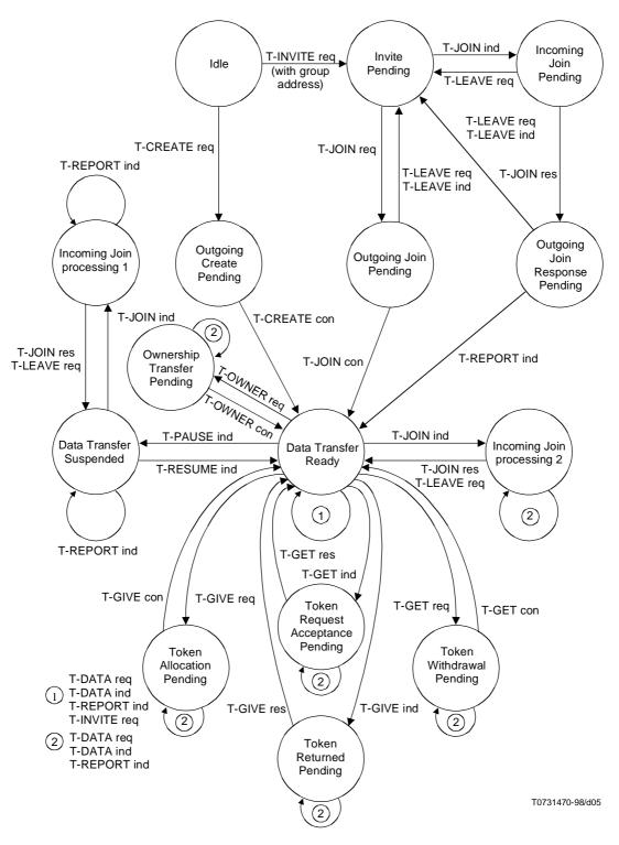
NOTE – T-TERMINATE request and/or indication may occur at any states, except the idle states, which then will lead to the Idle state. All states except the Data Transfer Suspended include a self-loop branch due to T-UNITDATA request and T-UNITDATA indication; these primitives may occur at such states without causing transition to other states.
