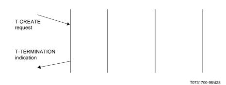
Figure 27 – Sequence of primitives in TS-provider rejection of a TC Creation attempt
