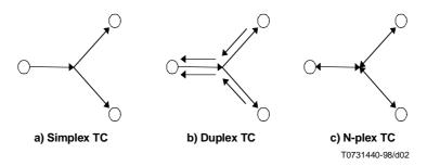
**Figure 1 – Types of Transport Connections**
