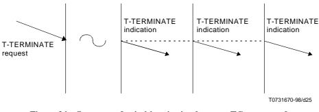
Figure 24 – Sequence of primitives in simultaneous TC-owner and TS-provider invocation of a TC termination
