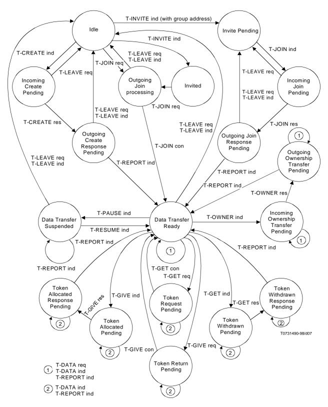
NOTE – T-TERMINATE request and/or indication may occur at any states, except the idle states, which then will lead to the Idle state. All states except the Data Transfer Suspended include a self-loop branch due to T-UNITDATA request and T-UNITDATA indication; these primitives may occur at such states without causing transition to other states.
