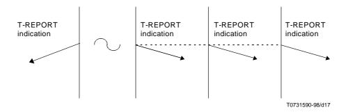
Figure 16 – Sequence of primitives during data transfer when the TS-provider is to give warning or notification
