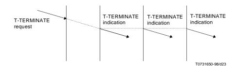
Figure 22 – Sequence of primitives in a TC-owner invocation of a TC termination
