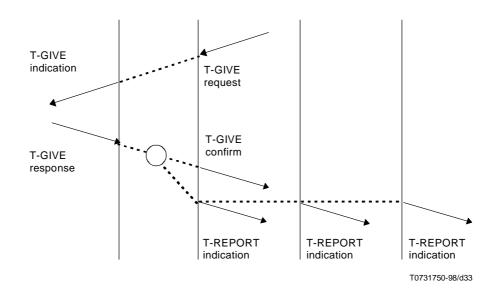
Figure 32 – Sequence of primitives in a token return to a TC-owner from a specified TS-user
