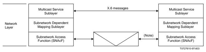
NOTE - Internal protocol in case the server is inside the network or SNAcP in case the server is outside the network.
