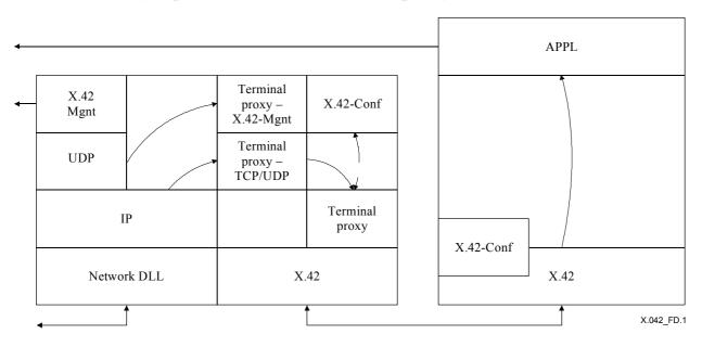
Figure D.1/X.42 – X.42 PAD with IP addressable terminals
