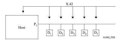
Figure 3/X.42 – GPAD minimum architecture – Traditional multipoint
