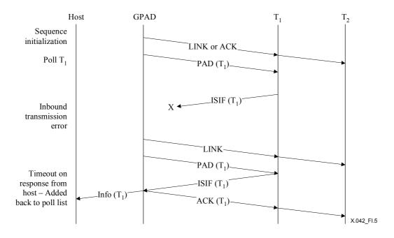
Figure I.5/X.42 – Solicited inbound transmission error
