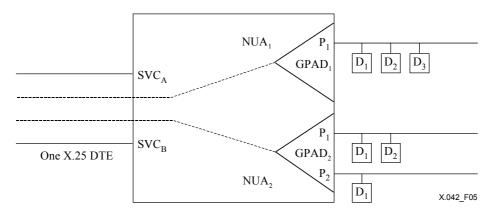
Figure 5/X.42 – PAD expanded configuration – Two GPAD instances
