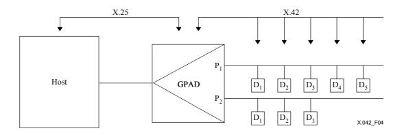
Figure 4/X.42 – GPAD minimum architecture – Networked implementation
