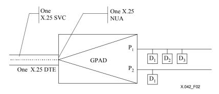
Figure 2/X.42 – GPAD minimal configuration
