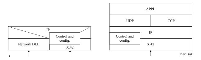
Figure 7/X.42 – Internal organization of GPAD terminal IP-enabled; X.42 encapsulation mode procedure class
