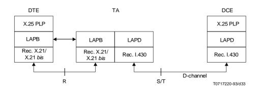
$FIGURE\ \ IV.2/X.31$  Example configuration in the idle phase, transparent at layer 3
