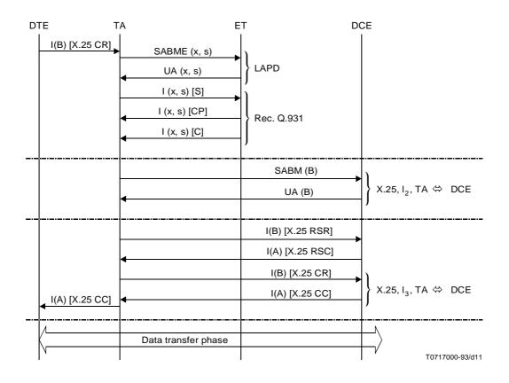
$FIGURE\ I.4/X.31$  Example Q.931 and X.25 message sequences for the establishment phase
