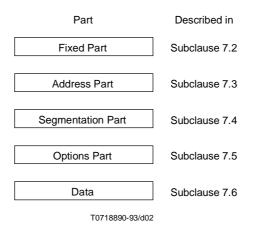
Figure 1 – PDU structure
