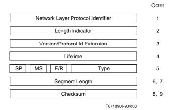
Figure 2 – PDU header – Fixed part
