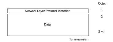
Figure 10 – Inactive Network Layer Protocol PDU
