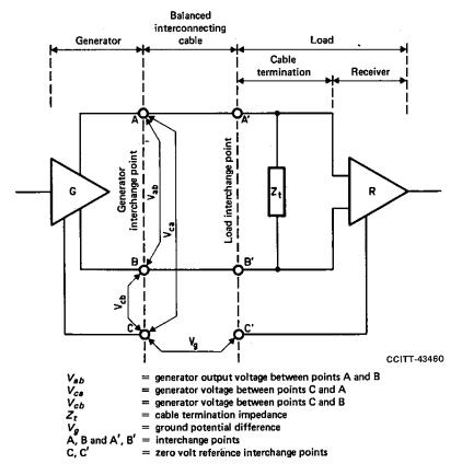
Note I – Two interchange points are shown. The output characteristics of the generator, excluding any interconnecting cable, are defined at the "generator interchange point". The electrical characteristics to which the receiver must respond are defined at the "load interchange point".
