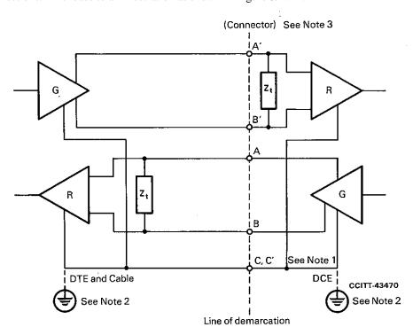
Note 1 - The zero volt reference interchange point C, C' may be interconnected via the signal ground conductor.
