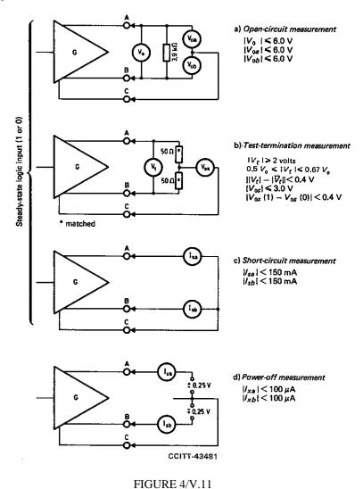
Generator-parameter reference measurements
