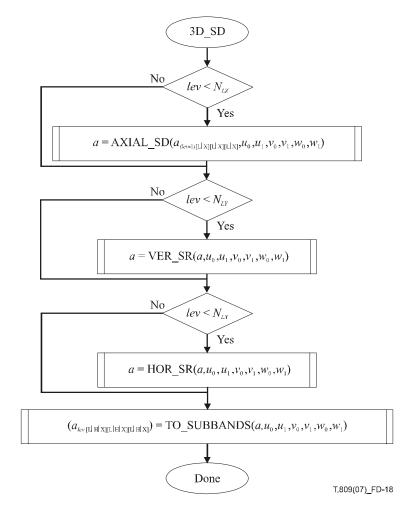
Figure D.18 – The 3D\_SD procedure
