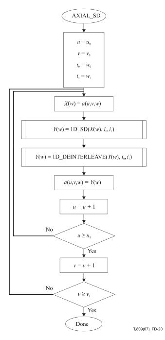
Figure D.20 – The AXIAL\_SD procedure
