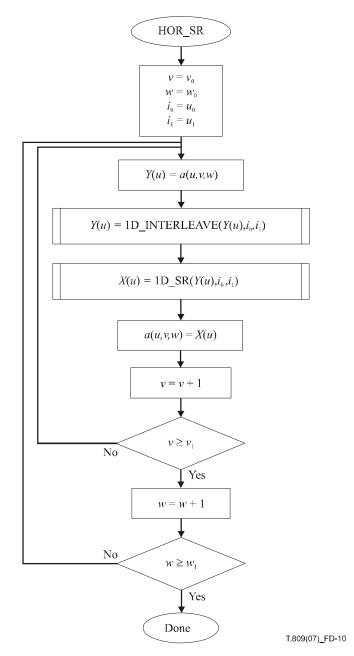
Figure D.10 – The HOR\_SR procedure
