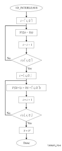
Figure D.8 – The 1D\_INTERLEAVE procedure
