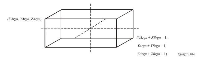
Figure E.1 – Cuboid mask on the reference grid
