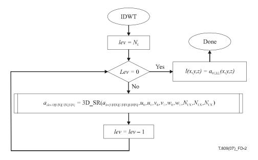
Figure D.2 – The IDWT procedure
