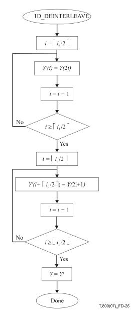
Figure D.26 – The 1D\_DEINTERLEAVE procedure
