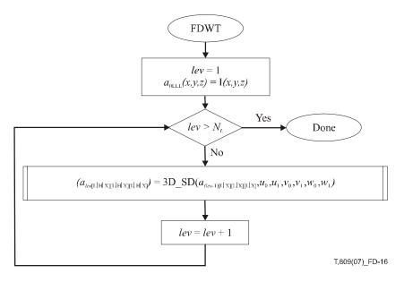
Figure D.16 – The FDWT procedure
