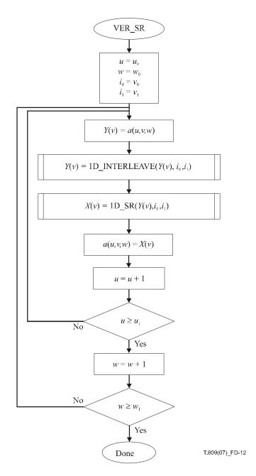
Figure D.12 – The VER\_SR procedure
