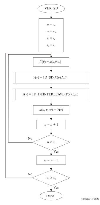
Figure D.22 – The VER SD procedure
