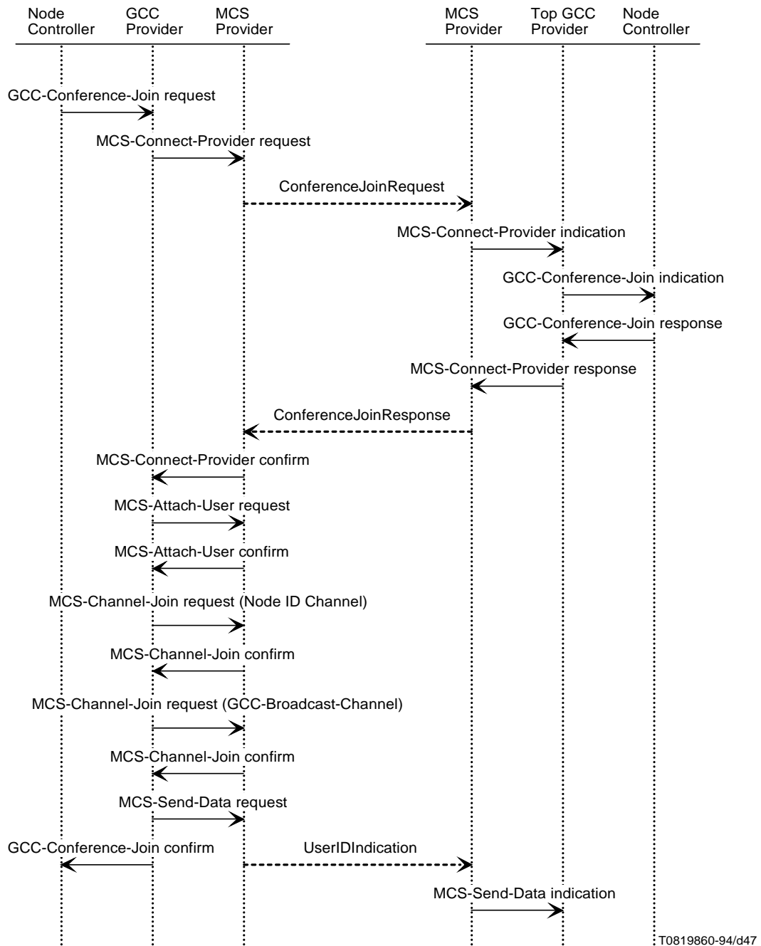
FIGURE 8-2/T.124 Joining a conference when directly connected to Top GCC Provider
